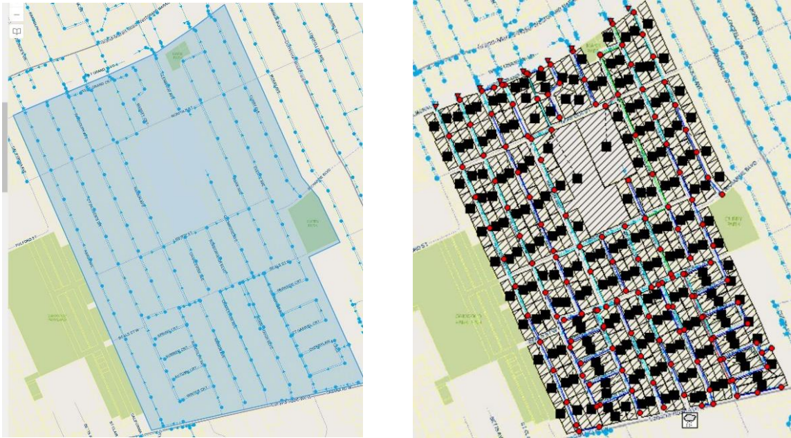
Figure 19- Stormwater Management Area and Model
