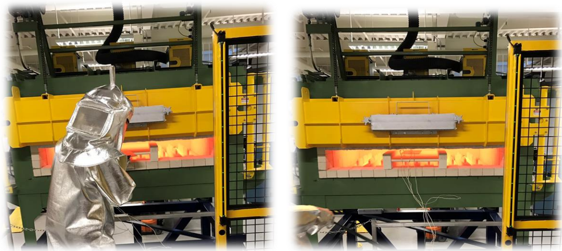
Figure 23 Removing blanks from the furnace using the main door
