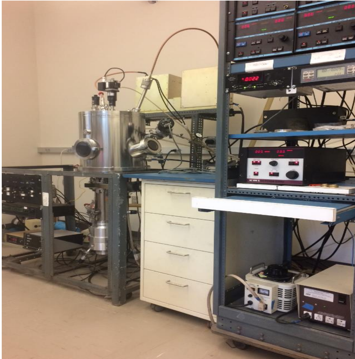
Figure 3.1: The reactive magnetron sputter deposition system used in this research.
