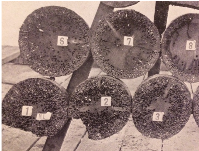
Figure 4: “Honeycombed” Timber: Credit: The San Francisco Marine Piling Committee of the American Wood-Preservers’ Association, Inc. [First] Report on the San Francisco Bay Marine Piling Survey, plate 2. Used with permission of the American Wood-Preservers Association.
