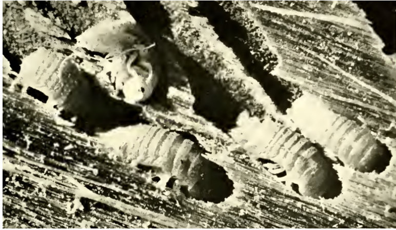
Figure 28: Limnoria Eating. The San Francisco Marine Piling Committee of the American Wood-Preservers’ Association, Inc. Final Report of the San Francisco Bay Marine Piling Committee , 319. Used with permission of the American Wood-Preservers Association.
