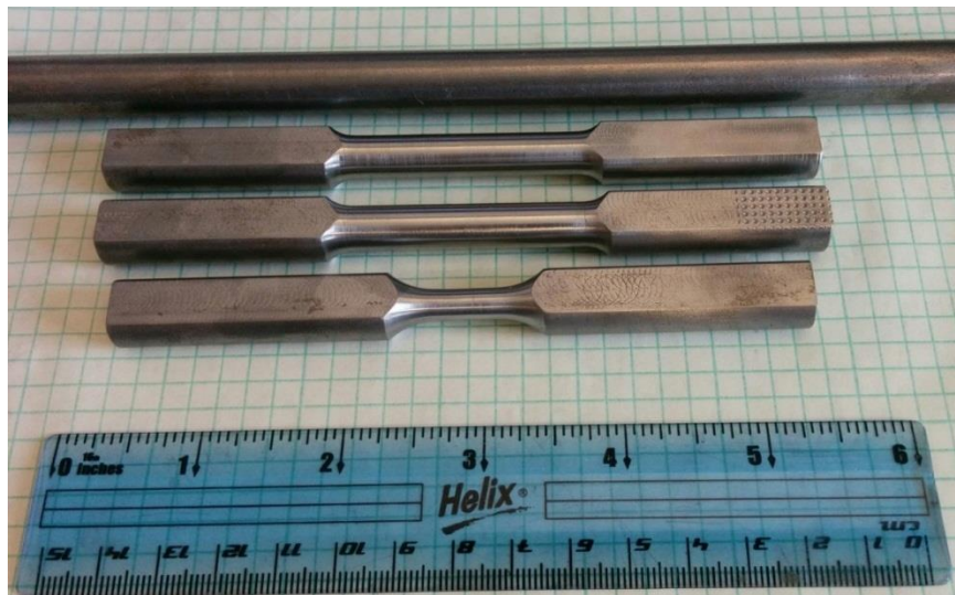
Figure III.4. Steel tension and LCF specimens for preliminary testing.
