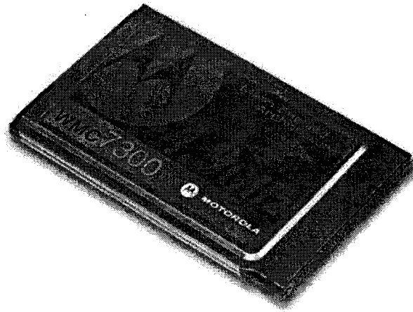
Figure 3.12. Motorola WMC7300 public safety 4.9GHz band MEA radio modem card for a notebook computer.
