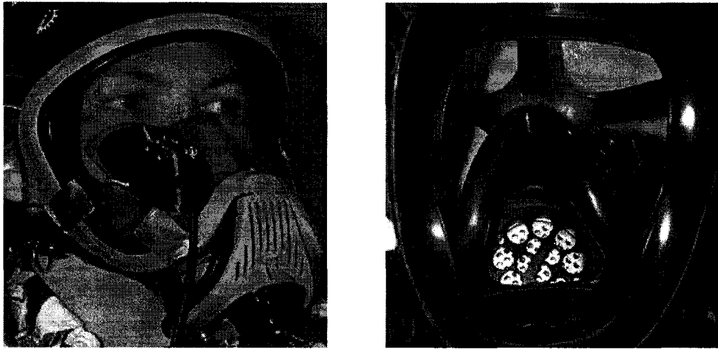
Figure 1.2 Prototype Head Mounted Display embedded within a Drager firefighter's mask. Left: External view, right: inside of mask. The coin-sized visor allows viewing downscaled floorplans. Source: [Wilson05]
