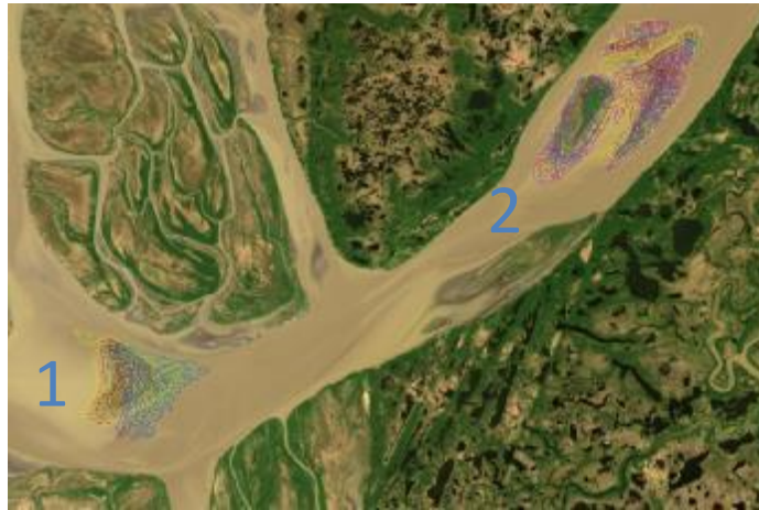
Figure 4.5. Two shallow-water sites in the Yukon River in which features were extracted using Canny edge detection.
