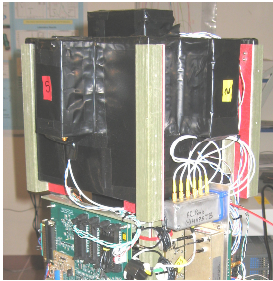
Figure 3.8: FACTEL Anti-Coincidence panels box around the D1 detector layer, see text for a description
