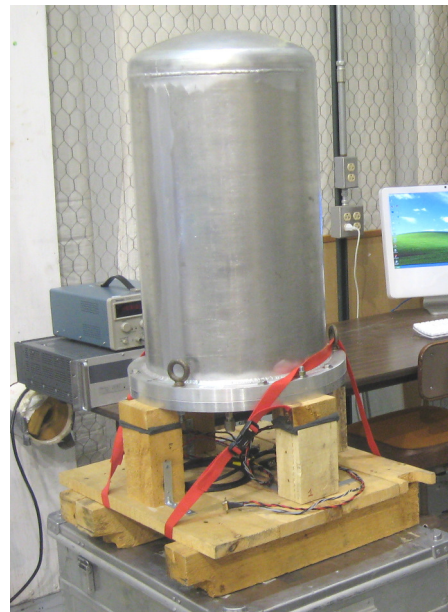
Figure 3.12: The FACTEL prototype pressure vessel
