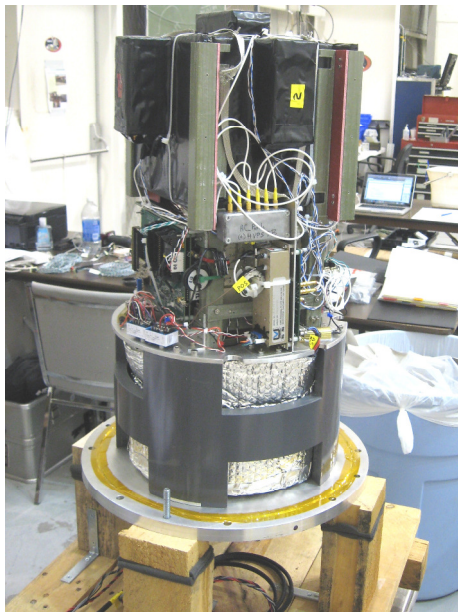
Figure 3.11: The assembled FACTEL prototype prior to the balloon flight
