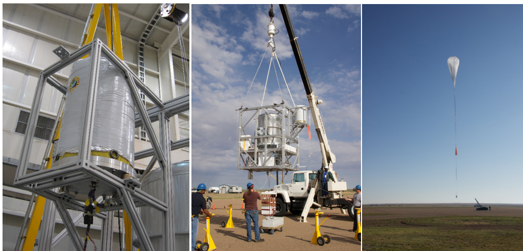
Figure 5.2: The FACTEL instrument mounted in its gondola frame (left), the GRAPE/FACTEL gondola (middle), the balloon launch (right)
