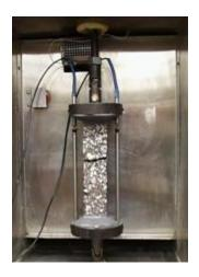
**Figure 2.9:** Sample TSRST setup (Asphalt Research Consortium, 2007)
