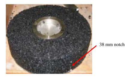
**Figure 2.11:** Asphalt Concrete Cracking Device setup (Kim, Sargand, and Wargo, 2009)
