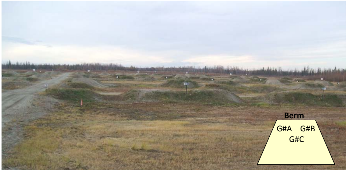
Figure 2-1. The small-arms Range 16 Records Range berms at Fort Wainwright. The inset shows where the grab samples were collected from at each of the 16 berms (G = grab sample; # = sample number, A, B, C = location on berm face).
