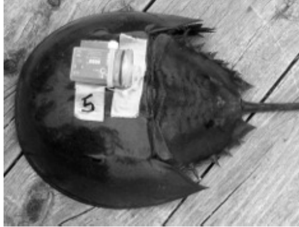
Figure 2.2. HOBO accelerometer attachment on dorsal carapace of individual horseshoe crab (photo credit: Win Watson).
