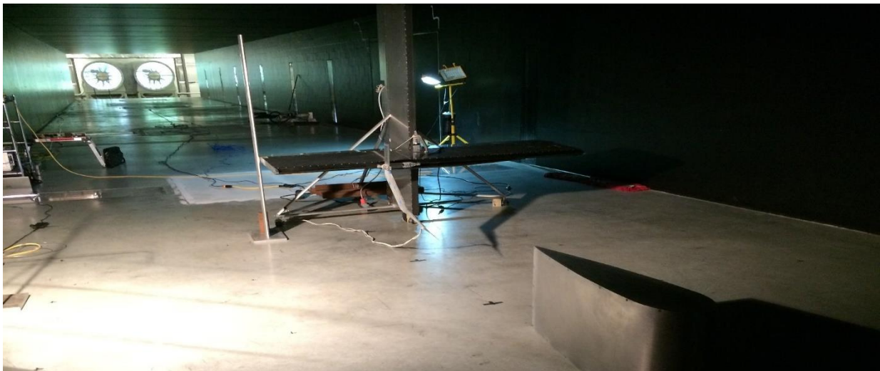
Figure 2.4.4: Final experiment setup including: airfoil, 2D traverse, hot-wire probe, and computer system in the UNH FPF
