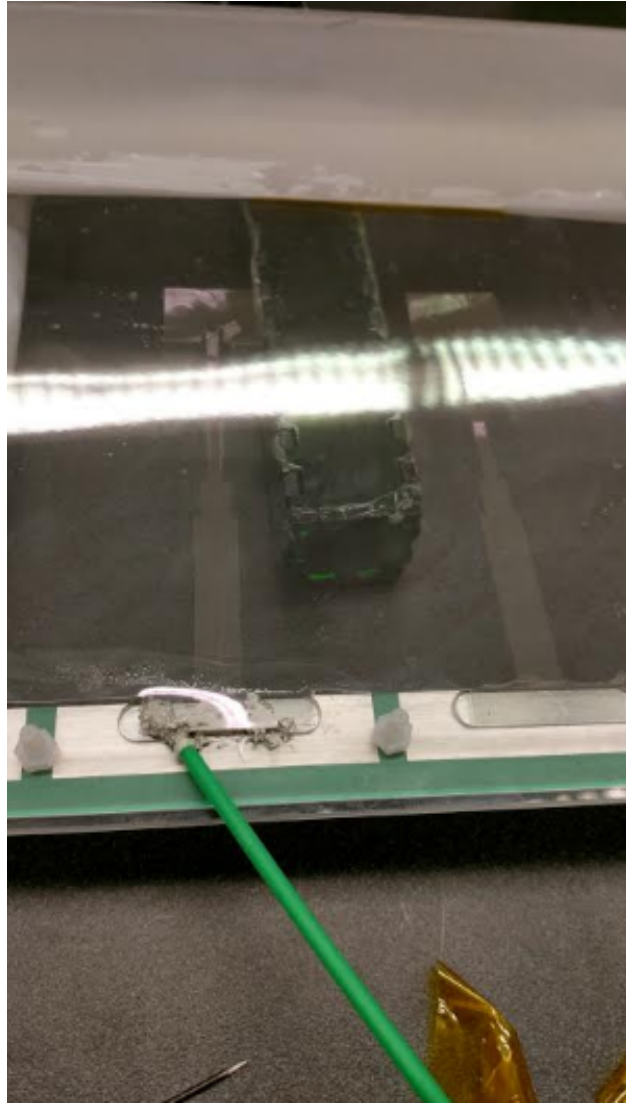
Figure A.29: Creating electrical continuity between the edge board and the ground plane using silver epoxy.
