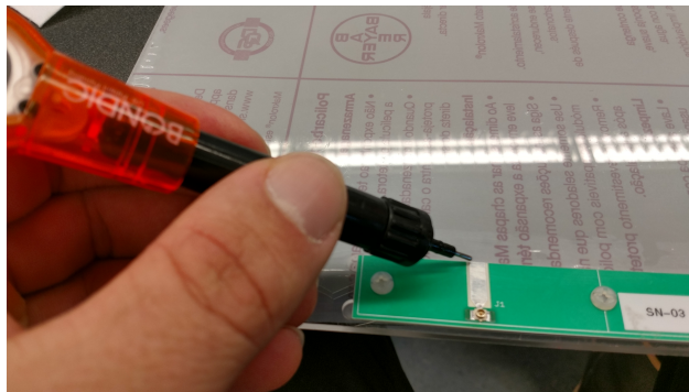
Figure A.10: Ensuring isolation from the patch side of the antenna and the ground side of the antenna.
