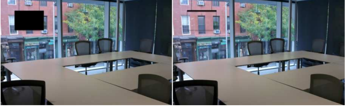
Figure 1.2: Comparing the obtrusiveness of an opaque antenna to a transparent antenna mounted in a window [2].
