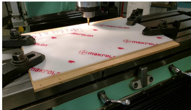
Figure A.5: Lexan board sitting in milling workspace.
