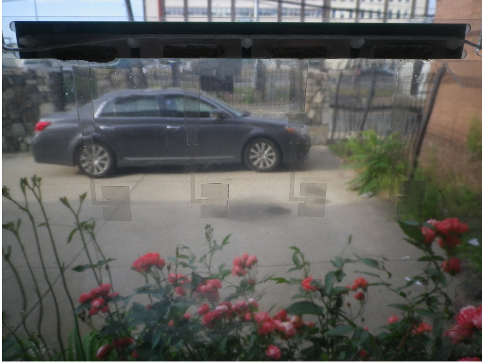
Figure B.2: Deployed horizontally-polarized transparent antenna array.
