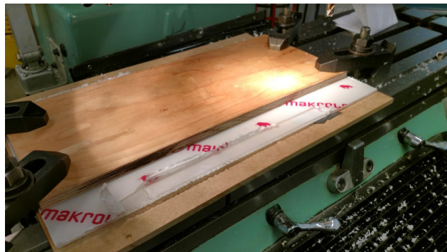
Figure A.6: Lexan board cut on milling machine.
