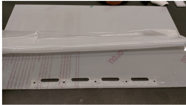
Figure A.7: Showing the cut into the Lexan made by the milling machine.
