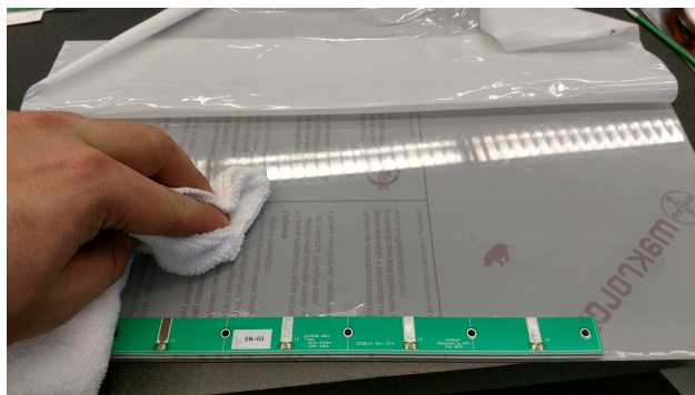
Figure A.11: Cleaning the surface where the patch antennas will be attached.
