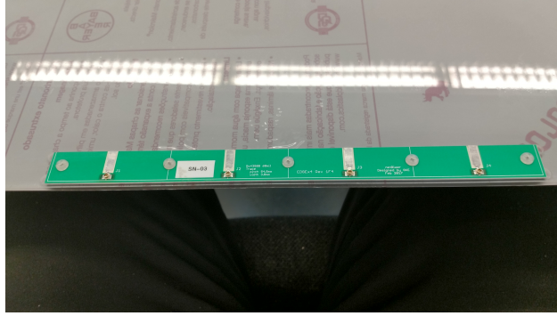
Figure A.9: Edge board placed into milled lexan.
