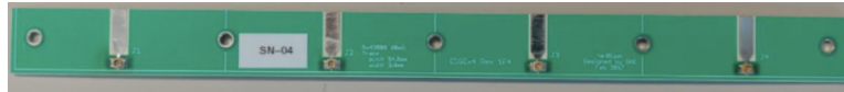
Figure 4.2: Edge board used to electrically connect transparent hardware to Butler matrix with UMCC connectors.
