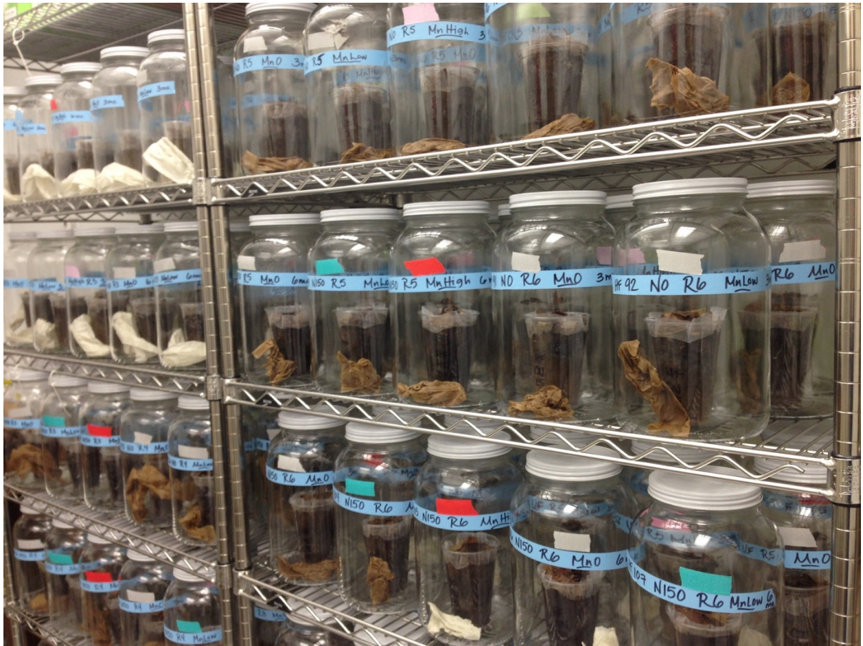
Photo 2. Incubation jars in the environmental chamber (25°C). Sealed glass pickle jars with wetted paper towels were used to maintain soil and litter moisture. Large pickle jars were selected to maximize headspace, thus minimizing the times jars needed to be aerated.
