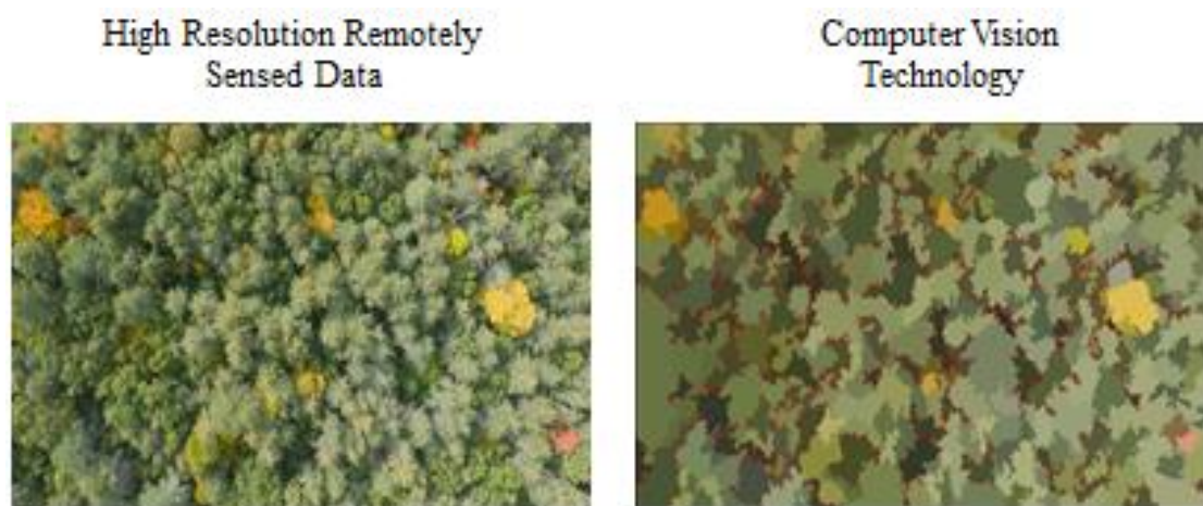
Figure 3. Computer Vision Interpretation Mimicry of the Human Ocular System, segmentation processed by Trimble eCognition Developer v9.2.0.
