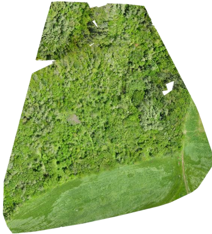
Figure 22. Orthomosaic result for 50m above canopy flying height, captured with the SODA.
