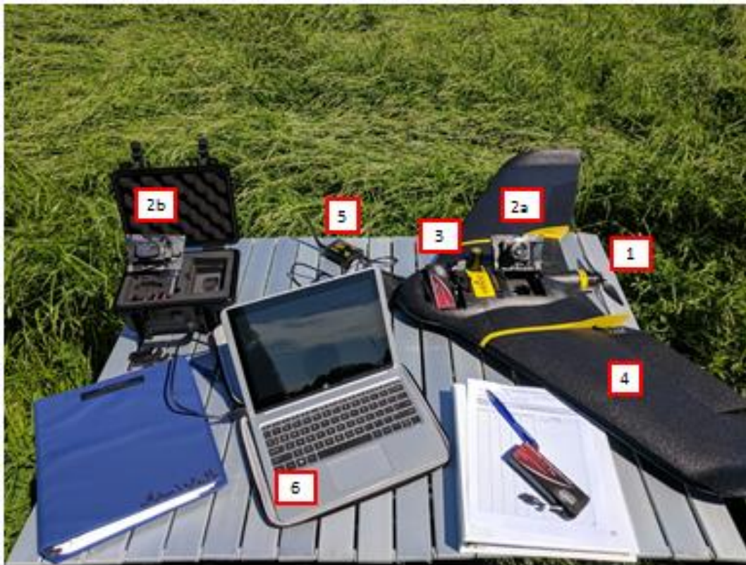
Figure 12. eBee Plus system configuration with (1) flight mechanism, (2a) SODA and (2b) sequoia payloads, (3) battery, (4) aircraft, (5) communication link, (6) ground control software and controller. Also pictured are the hardware and software manuals, in color (far left).
