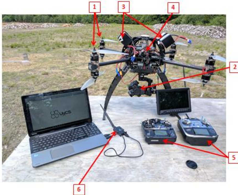
Figure 11. Aeronavics Skyjib X-8 complete system configuration including: (1) eight-rotor flight mechanisms, (2) Panasonic GH4 payload, (3) two Tattu battery placements, (4) unmanned aircraft, (5) 2 manual command and control elements, one for aircraft, one for gimbal, and (6) Bluetooth communication data link for laptop. Also pictured are the FPV monitor (right, under drone) and UGCs mission planner (left).
