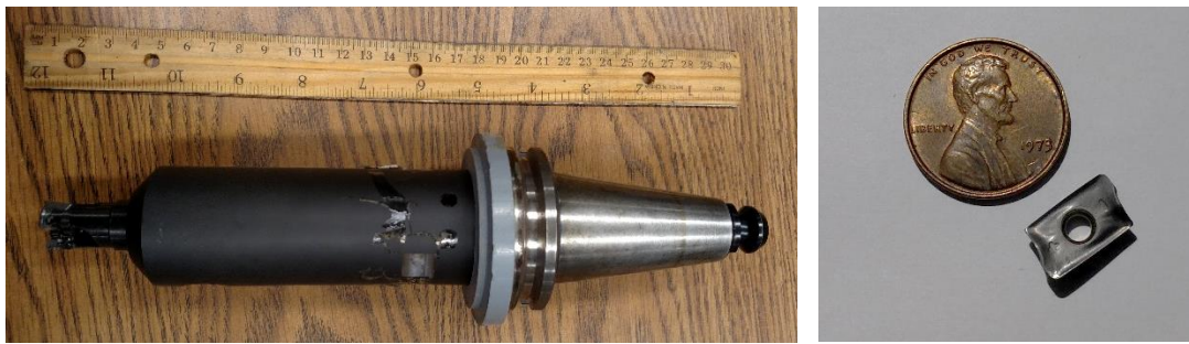
Figure 34: Cutting tool used for experimental cuts (left). Sandvik Carbide insert (right).
