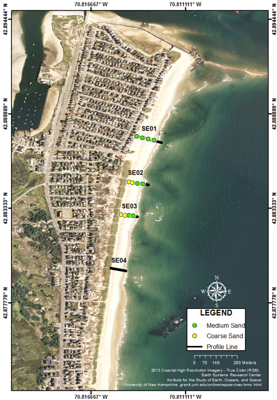
Figure 5-26: Location map of stations on Seabrook Beach, New Hampshire. Black lines are the profile locations while dots represent summer 2015 sediment sample locations. Sediment size classification (after Wentworth, 1922) is shown by dot color. The profile line without sediment information was established after summer 2015 sediment sampling.
