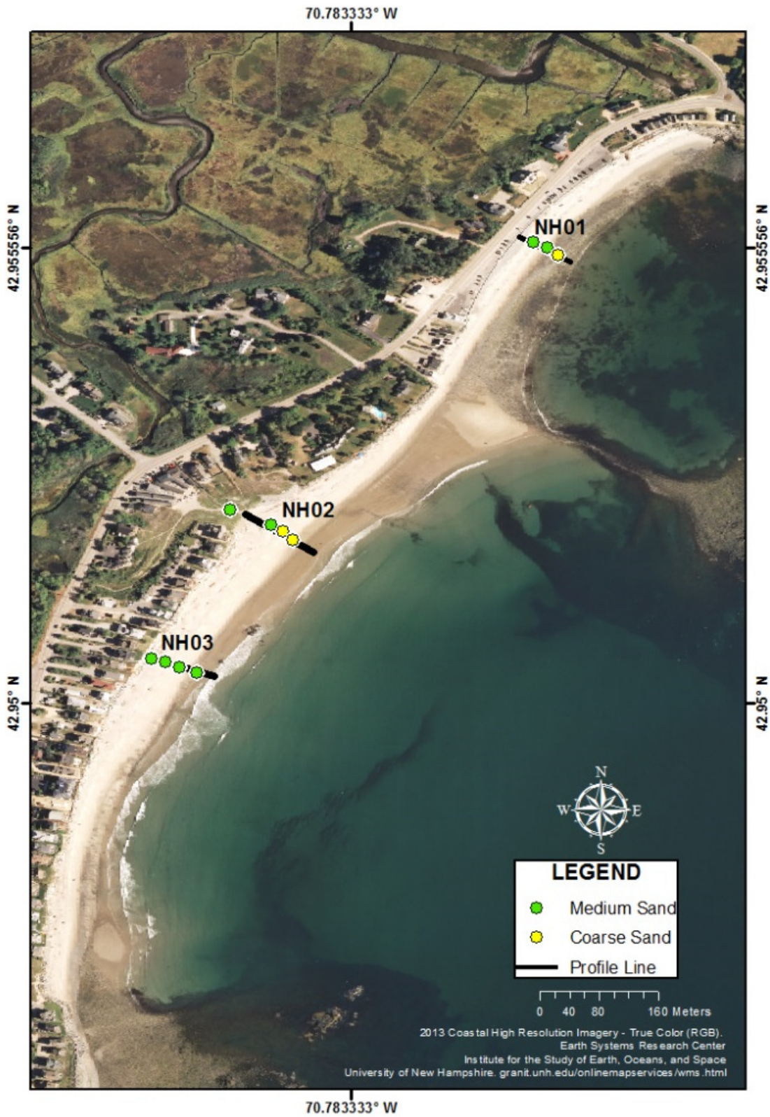
Figure 5-16: Location map of stations on North Hampton Beach, New Hampshire. Black lines are the profile locations while dots represent summer 2015 sediment sample locations. Sediment size classification (after Wentworth, 1922) is shown by dot color.
