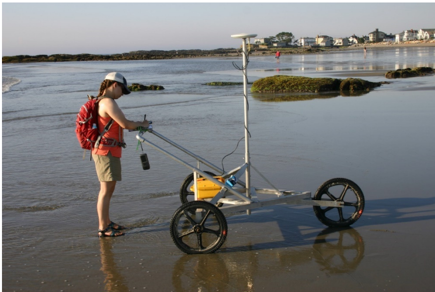
Figure 3-2: A beach profile being measured using the GNSS rover method at Wallis Sands on 08/03/15.
