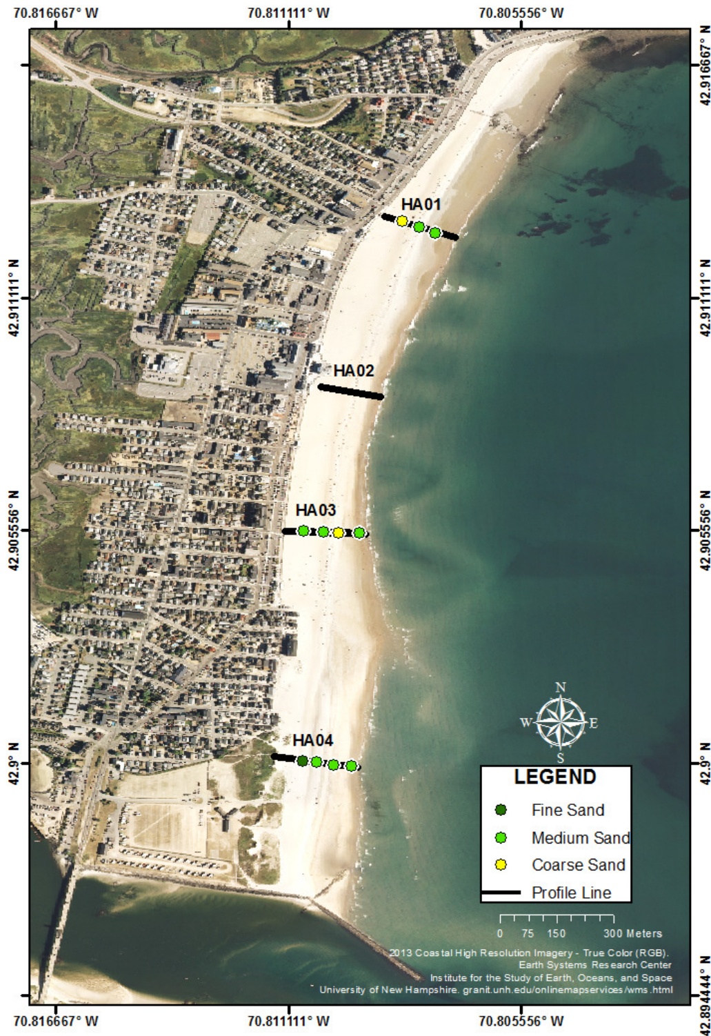
Figure 5-21: Location map of stations on Hampton Beach, New Hampshire. Black lines are the profile locations while dots represent summer 2015 sediment sample locations. Sediment size classification (after Wentworth, 1922) is shown by dot color. The profile without sediment information was established after the summer 2015 sediment sampling.
