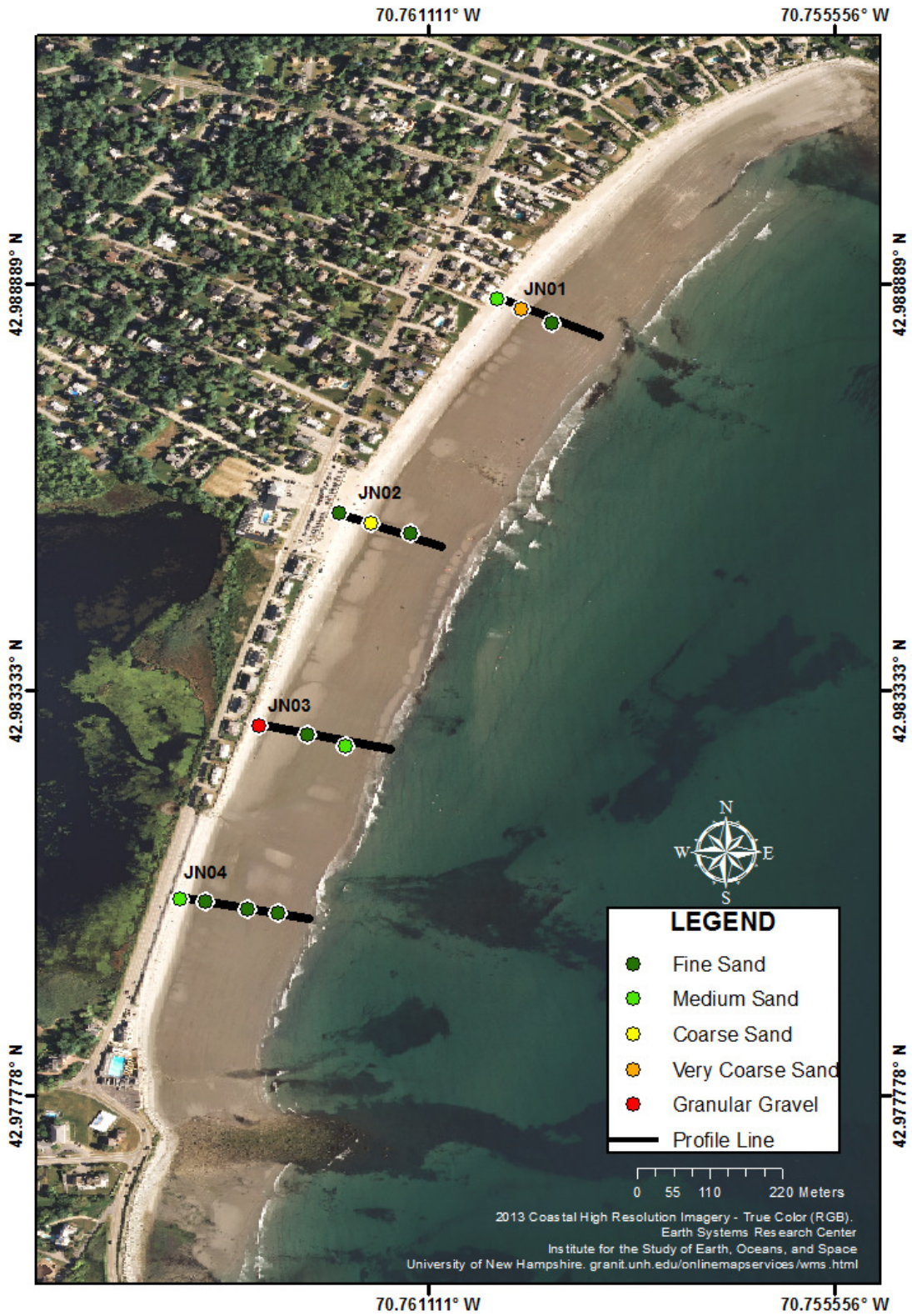
Figure 5-11: Location map of stations on Jenness Beach, New Hampshire. Black lines are the profile locations while dots represent summer 2015 sediment sample locations. Sediment size classification (after Wentworth, 1922) is shown by dot color.
