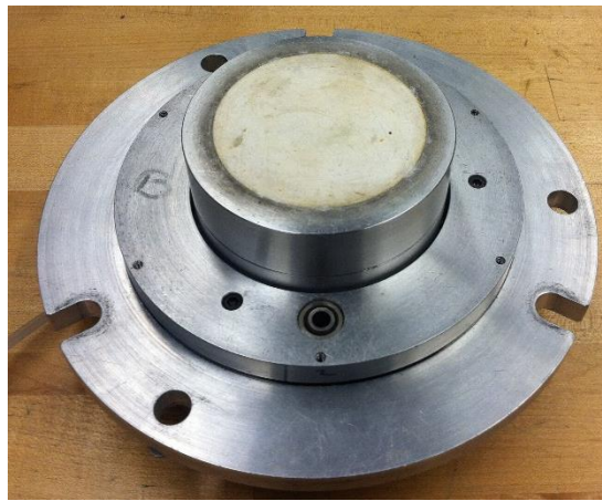
Figure 25: Modified Base Platen w/ embedded HAEV ceramic disk
