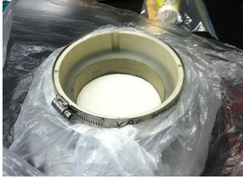
Figure D10: Soil Sample prepared for Sand Pluviation
