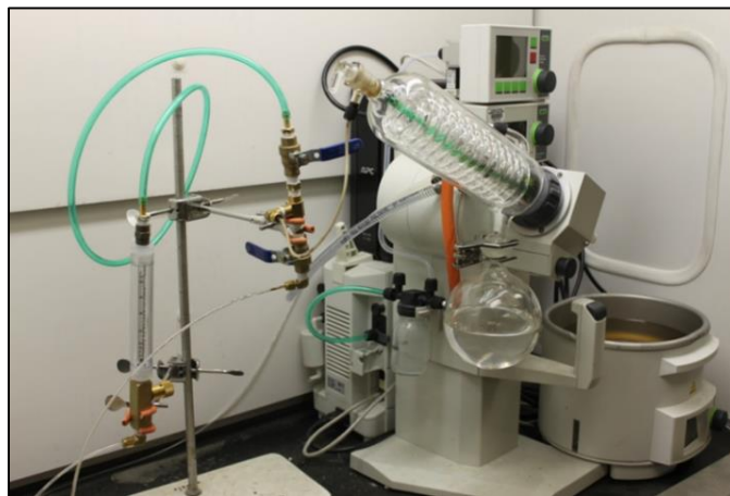
Figure 5: Rotary Evaporator System at Rutgers University for Asphalt Binder Recovery
