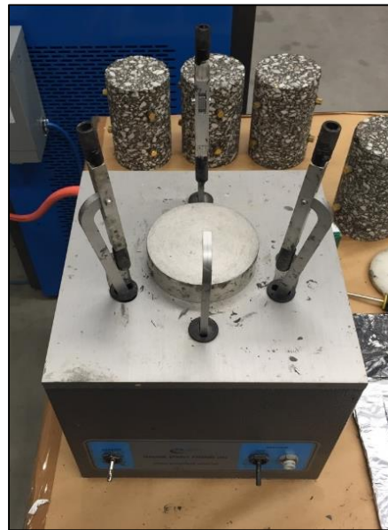
Figure 6: Gluing Jig Apparatus for Applying Studs
