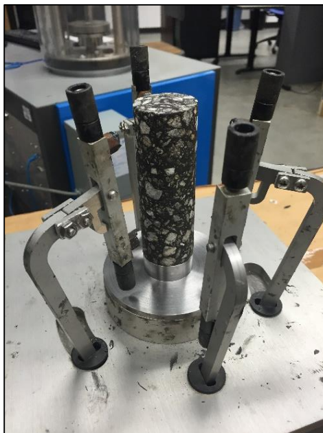
Figure 13: Gluing Jig Apparatus for Applying Studs to Small Specimens
