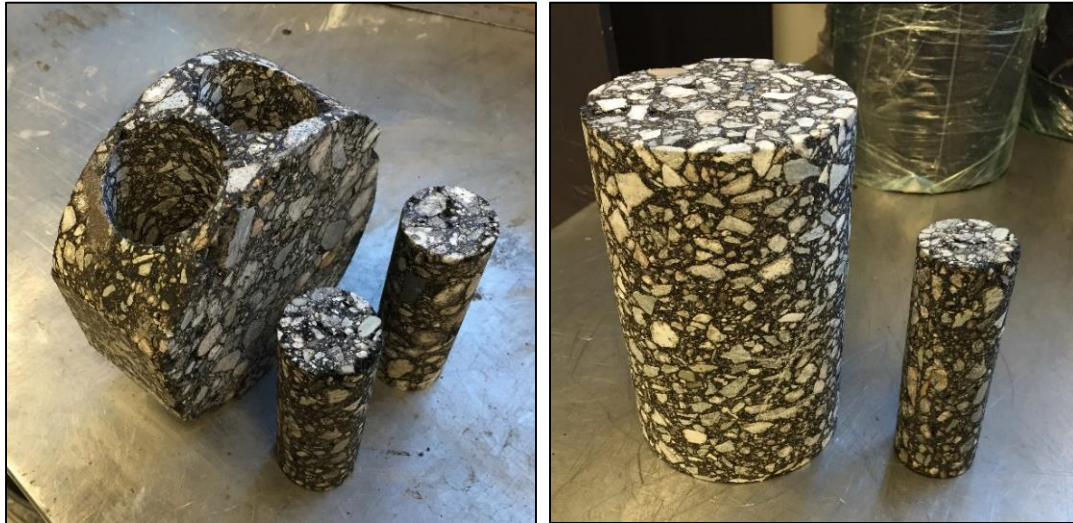
Figure 12: Two Small Specimens Produced from Field Core (Left) and Comparison with Standard Size Geometry (Right)
