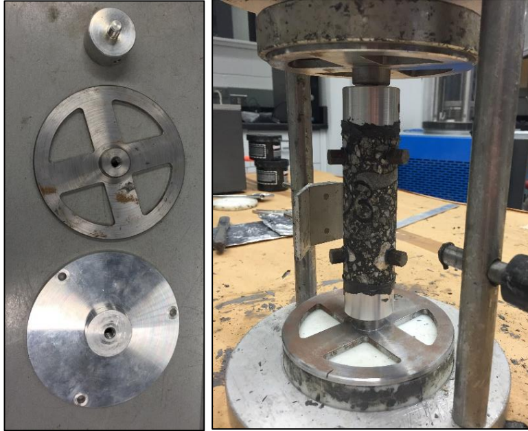
Figure 14: Machined Parts and Gluing Jig for Small Specimen S-VECD Fatigue Testing
