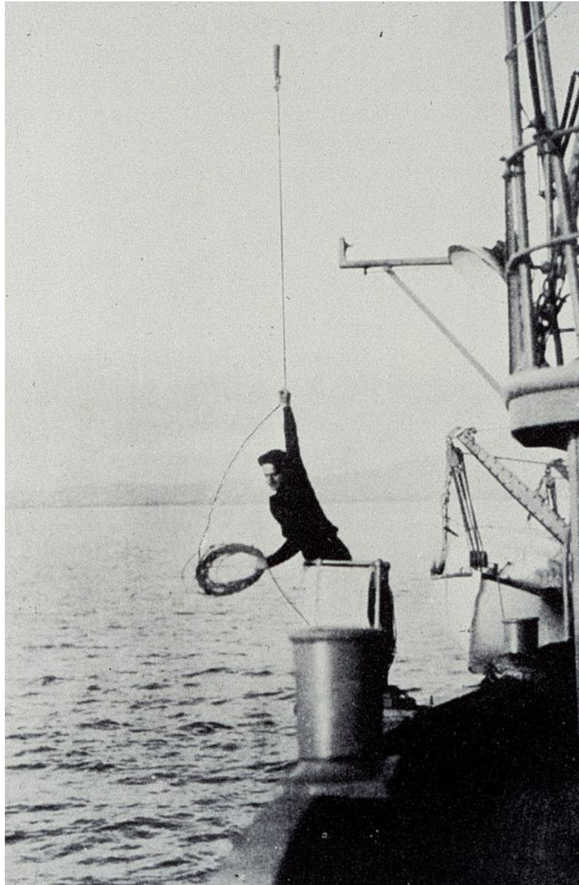
Figure 2: Use of a lead line ( www.noaa.gov )
