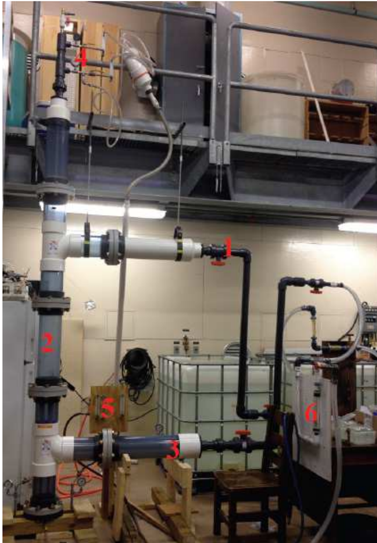
Figure 2.7 Vertical diffused aeration apparatus, where 1) is the influent water piping, 2) is the main reactor column, 3) is the effluent water piping, 4) are the air release valves and effluent airflow monitoring, 5) is the pressure and air inflow monitoring, and 6) is the flow meter
