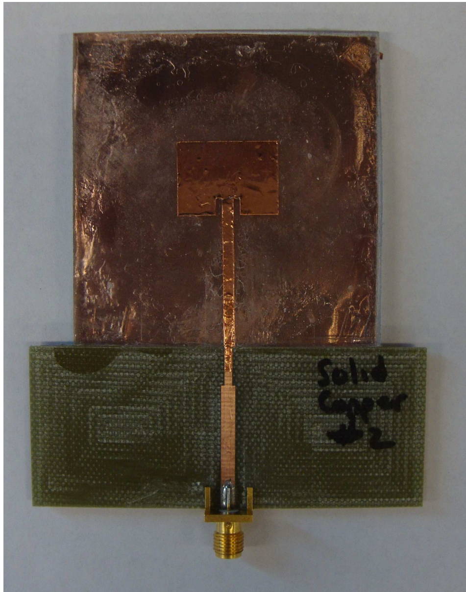
Figure A.1: Fabricated solid copper antenna over a solid copper ground plane
