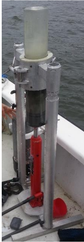
Figure 8 An aluminum frame held a core in place while a hydraulic jack was used to slowly push the core upward until exactly 2 cm were exposed.
