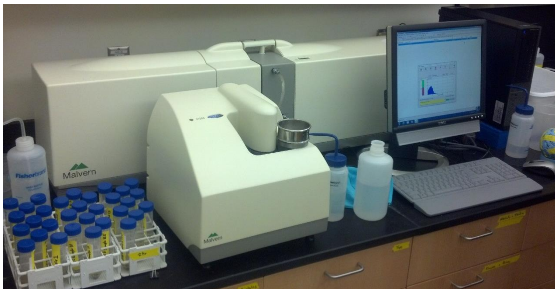
Figure 9 The Malvern Mastersizer laser diffraction size analyzer used to measure the size distribution of sediment samples.
