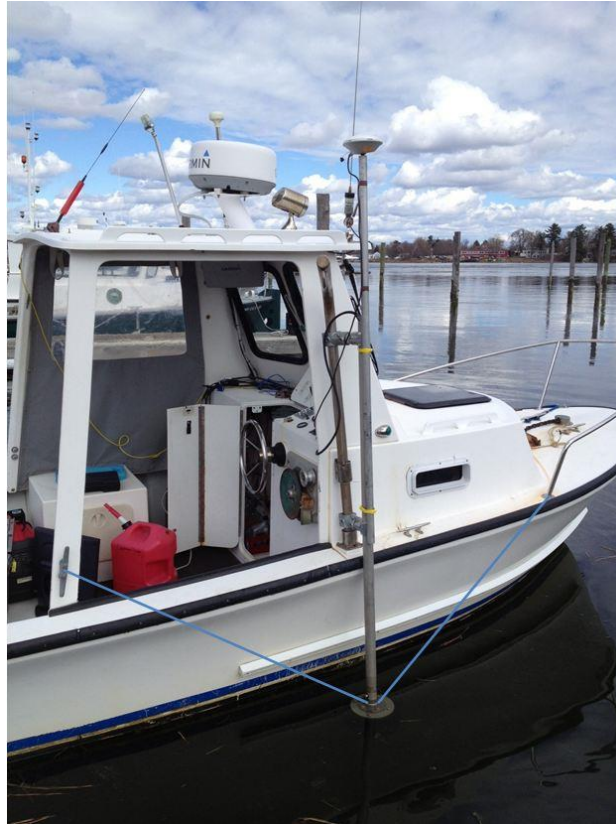
Figure 3 The R/V Galen J, a 22 foot open-cabin vessel used for surveying with the airmar transducer pole mounted to the starboard side with straps to stabilize the transducer head. A GPS receiver is mounted to the top of the transducer pole and a RTK receiver is mounted to the roof of the cabin.
