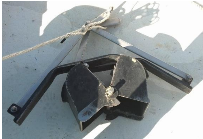
Figure 4 The gravity driven grab sampler used to collect surface sediment for grain size analysis
