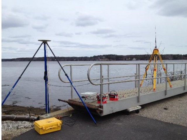
Figure 2 GPS Base Station set up at the Great Bay Marine. The RTK antenna (right) transmitted correction from the GPS receiver (left) to the boat.
