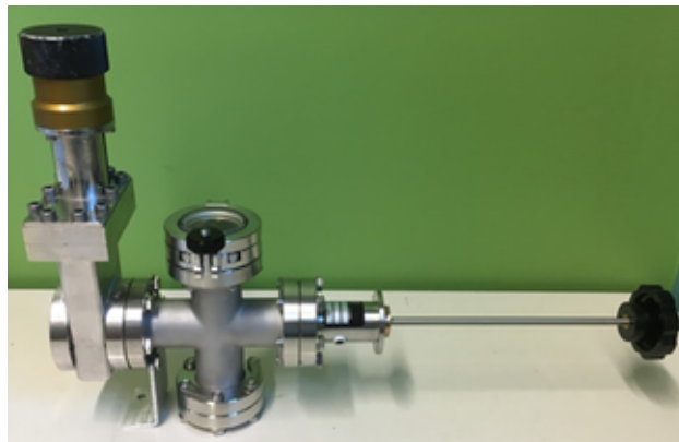
FIG. 14: This transit chamber helps us keep samples from touching atmosphere when being transferred from the glovebox to our UHV chamber. The end with the gate valve attaches directly to the back of the load lock.
