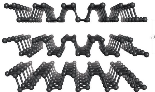
FIG. 1: A schematic of the structure of black phosphorus. Along the ridges is the zig-zag direction, and across them is termed the armchair direction. The mobility is greater in the armchair direction, reaching up to 10,000 \frac{cm^2}{Vs} [8].
