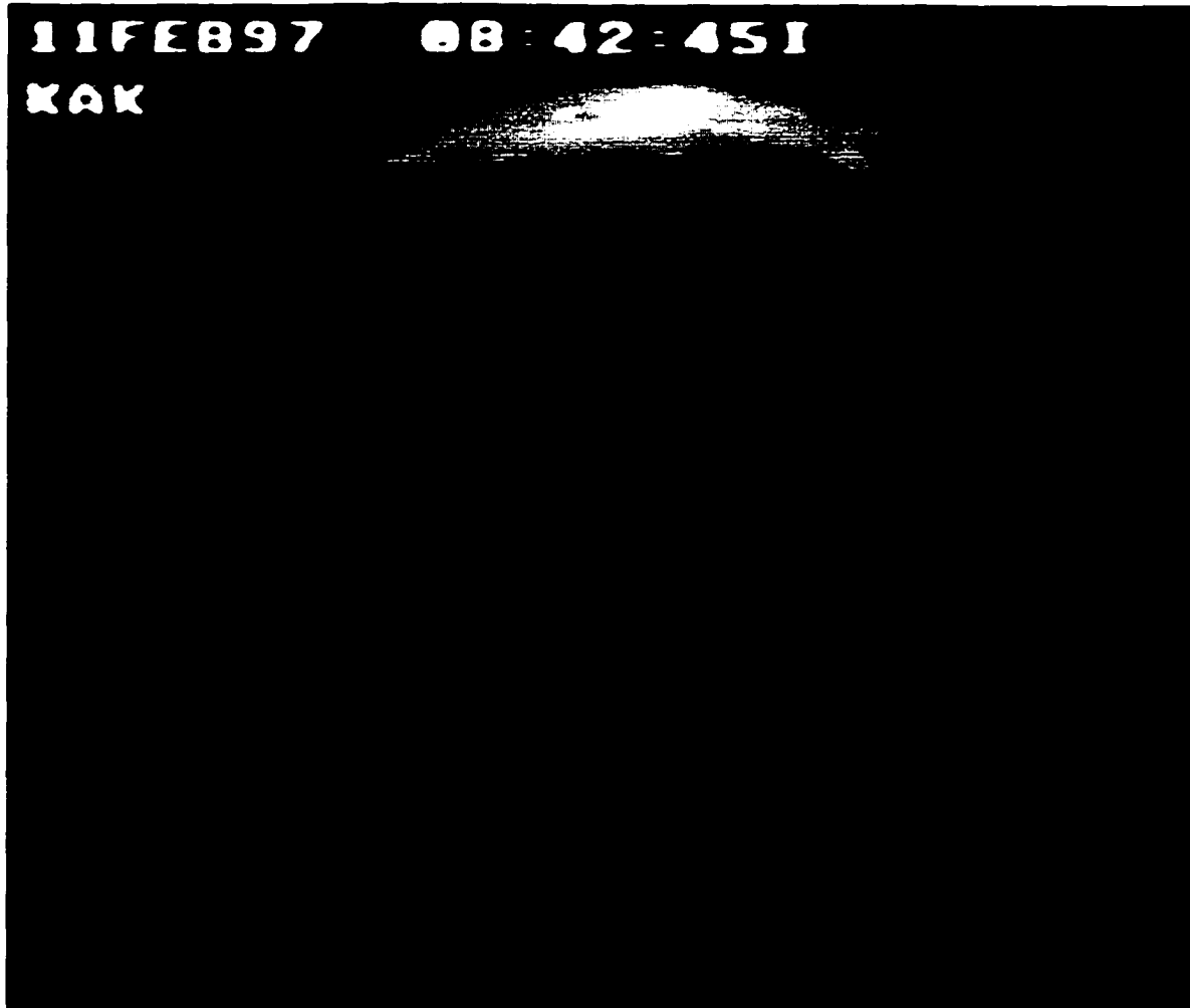
Figure 3-1: All-sky image from Kaktovik during the flight (T+365 seconds). The bright dot in the image is an enhanced pixel representing the location of the three payloads.
