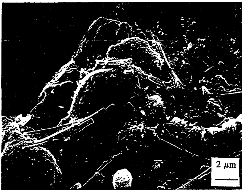
Figure 9.12 < No.200 Bottom Ash (SEM Photograph)
