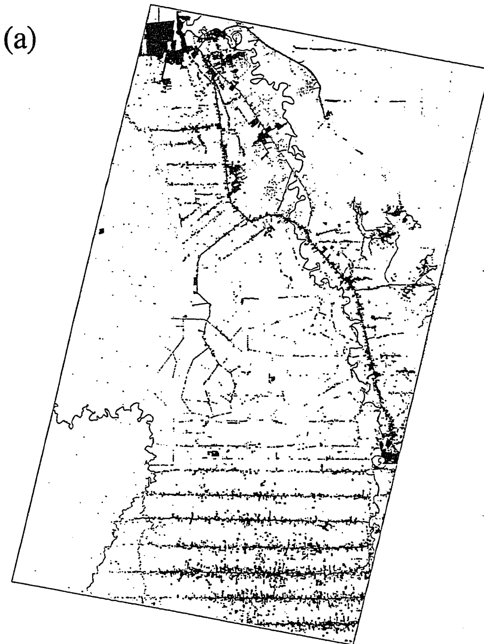
Figure 4.2. Results from a simple forest-deforested classification for each remote sensing method analyzed in this study: (a) SPOT 20m multispectral data classified using digital image processing and a maximum likelihood statistical classifier, (b) Landsat Thematic Mapper 30m resolution multispectral data classified using digital image processing and a maximum likelihood classifier, (c) Landsat Thematic Mapper data from channel 5 produced as a 1:250,000 scale photographic product interpreted visually and encoded with vector GIS techniques, (d) AVHRR-LAC data classified using a maximum likelihood statistical classifier, and (e) AVHRR-LAC data classified using a channel 3 brightness temperature threshold.
