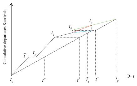
Figure 4.4. Equilibrium profile with capacity waste at only t<sup>-</sup>
