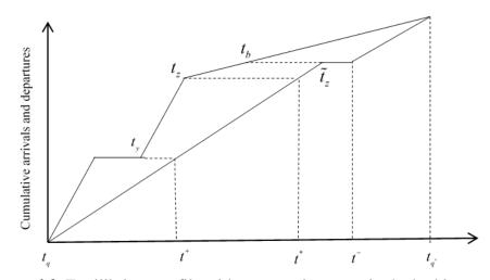
Figure 4.2. Equilibrium profile without capacity waste in the braking model
