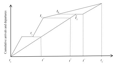
Figure 3.4. Equilibrium profile under coarse tolling: the braking model
