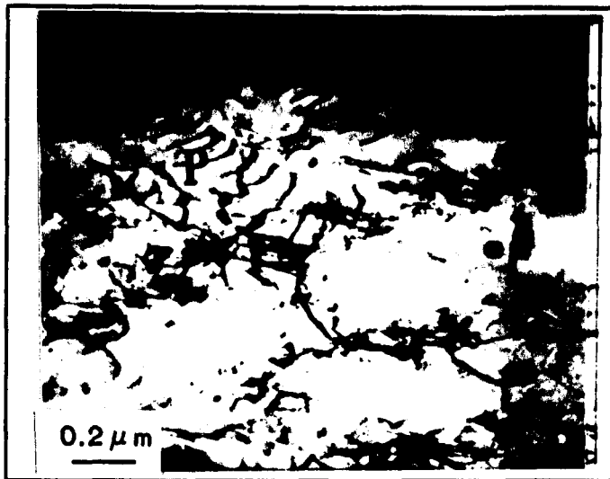
Figure 63 Microstructure of the BZ in an annealed stainless steel substrate.
