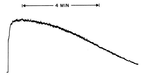
Figure 3-7. Photometer injection of 50  $\mu L$  of  $10^{-5}$   $\underline{M}$   $H_2O_2$  into 200  $\mu L$  of slower kinetics luminol-peroxidase reagent.
