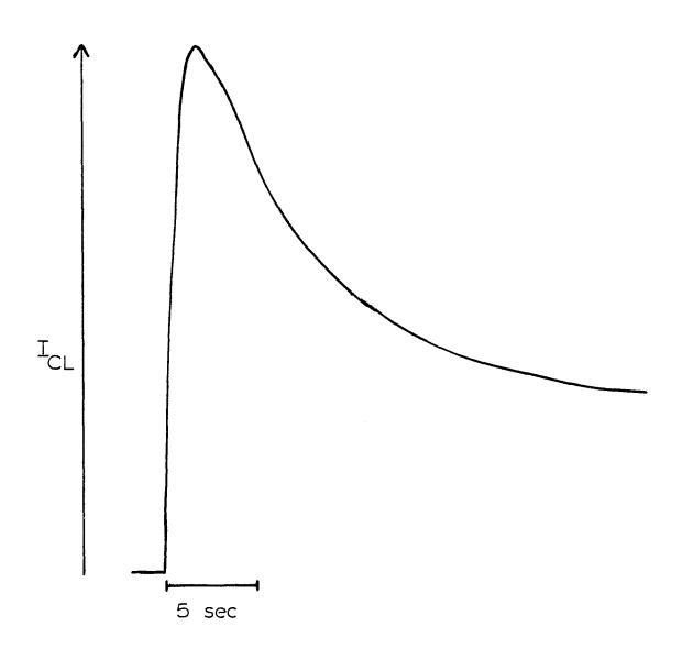
Figure 3-16. Photometer injection of approx. 100  $\mu L$  of  $10^{-5}$   $\underline{M}$  NADH into 100  $\mu L$  LUMASE bacterial BL reagent.
