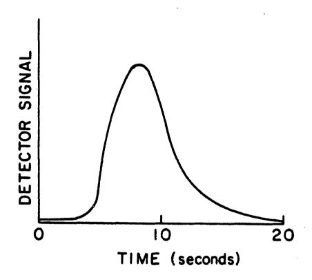
Figure 2-4. Typical FIA signal. The tailing is common for these systems.
