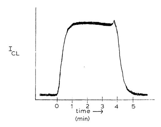
Figure 3-13. Steady state response of firefly system in two phase flow system with 10 mg/mL added apyrase. Flow rate = 1 mL/min.
