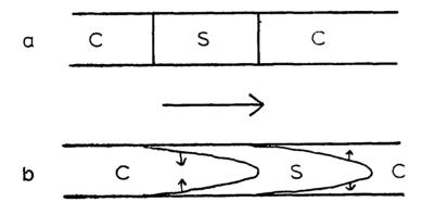
Figure 2-2. Development of parabolic concentration profile in a FIA system. Flow in the system is in the direction of the large arrow. (a) sample slug S when injected into carrier stream C; (b) concentration profile some time after injection; small arrows indicate radial diffusion.
