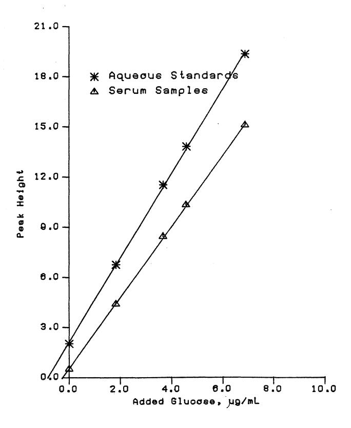
Figure 2-11. Standard additions curves for aqueous glucose solutions and serum standards. Difference in slopes of the lines indicates presence of an interference.
