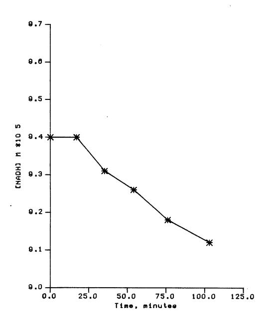
Figure 3-18. Plot showing degradation of NADH over time, as measured by absorbance at  $340\,\mathrm{nm}$ .
