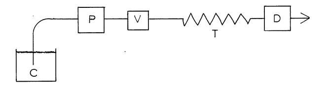
Figure 2-1. Components of a simple FIA system. C: carrier solution; P: pump; V: sample injection valve; T: tubing coil to enhance mixing; D: flow-through detector.
