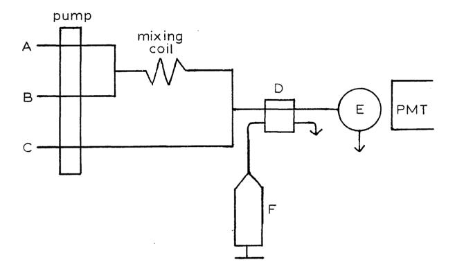
Figure 3-19. Final two phase flow system for bacterial BL. A: FMN solution; B: stirred decanal solution; C: NADH sample solution (or blank buffer); D: Rheodyne 4-way injection valve (for flow injection experiments); E: two phase flow cell; F: syringe for injection of sample (flow injection mode).
