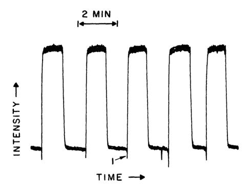
Figure 3-5. Steady state response for  $10^{-6}$  M  $_{2}^{0}$   $_{2}$  in the two phase flow system, using fast kinetics luminol-peroxidase reaction. Flow rate = 5 mL/min.
