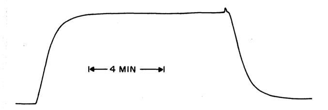
Figure 3-10. Steady state response of 1.6 x  $10^{-6}$  M ATP in two phase flow system. LUMIT reagent in the reagent cell contained 1 mg/mL added apprase. Flow rate =1 mL/min.
