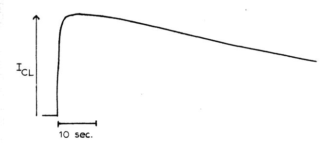
Figure 3-9. Photometer injection of 25  $\mu L$  of  $10^{-6}$  M ATP into 100  $\mu L$  of LUMIT firefly reagent with 1 mg/mL of added apyrase.
