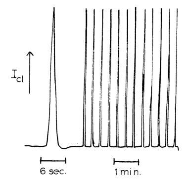
Figure 2-13. Typical data for glucose determination. Data shown are replicate injectons of a 0.85 µg/mL glucose solution. Intensity is on an arbitrary scale. The first peak was run at a high chart speed to show peak shape more clearly. The second set shows the type of data normally taken for analysis of peak height.
