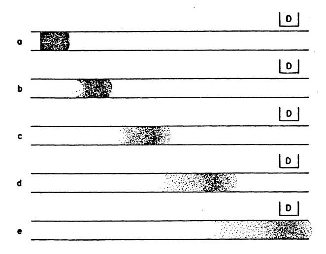
Figure 2-3. Dispersion of sample slug from injection (a) as the flowing stream proceeds down the tubing and past the detector D.
