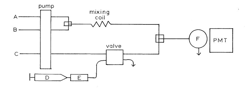
Figure 2-10. FIA system for Fe(CN)<sub>6</sub><sup>3-</sup>-catalyzed system for glucose determination. A: ferricyanide solution; B: luminol in boric acid buffer; C: acetate carrier buffer; D: sample solution; E: immobilized glucose oxidase column; F: tubing coil mounted in front of photomultipier. The pump for solutions A, B, and C is a 3-channel peristaltic pump. The sample (D) was pumped by a single-channel infusion pump.
