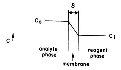
Figure 3-1. Schematic showing analyte concentration profile in ideal two phase flow cell. Co is analyte concentration in the bulk analyte phase. Ci is analyte concentration in the reagent phase.
