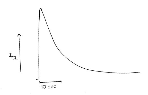
Figure 3-12. Photometer injection of  $10^{-6}$  M ATP using LUMIT reagent containing 10 mg/mL added apprase.
