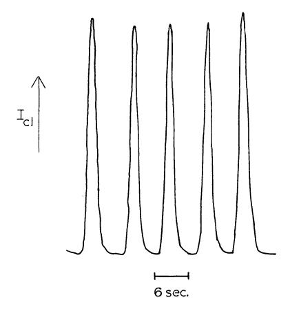
Figure 2-7. Replicate injections of  $10^{-6}$  M Cr<sup>3+</sup> in 0.4 M H<sub>2</sub>O<sub>2</sub>, titrated with KOH to pH 3-4.
