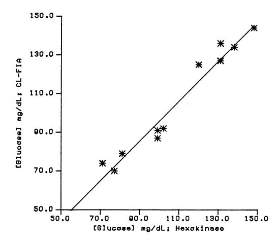
Figure 2-16. Results of a correlation study comparing results for blood glucose determination by CL-FIA and a reference method (Sigma glucose determination kit 15-UV).
