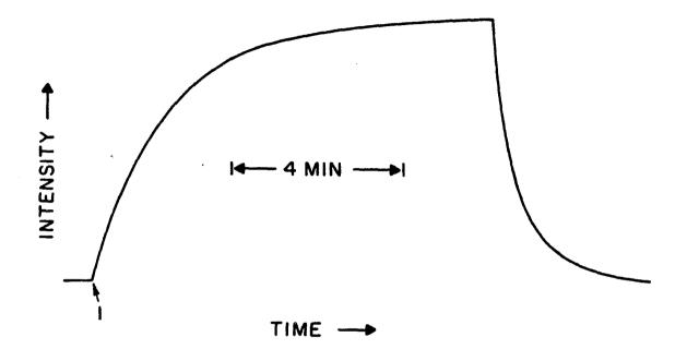
Figure 3-8. Steady state response of  $10^{-5}$  M  $\rm H_2O_2$  in slower kinetics luminol-peroxidase reaction in two phse flow system. Flow rate = 1 mL/min.
