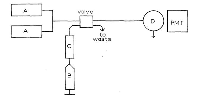
Figure 2-9. FIA system for Cu(II) catalyzed luminol system for glucose determination. A: luminol-Cu(II)-NH3 solution; B: sample solution; C: immobilized glucose oxidase column; D: tubing coil mounted in front of photomultiplier.
