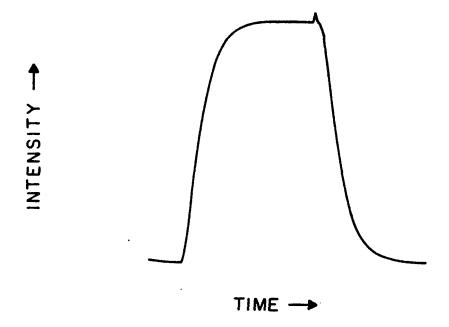
Figure 3-11. Steady state response for replicates of  $10^{-6}$  M ATP in two phase flow system with 1 mg/mL apyrase. Note the decrease in I<sub>SS</sub> from one replicate to the next. Flow rate = 1 mL/min.
