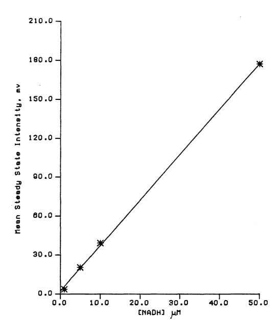
Figure 3-20. Standard curve for a limited number of NADH standards in the two phase flow system.
