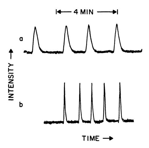
Figure 3-6. Replicate injections of  $10^{-6}~\underline{\text{M}}~\text{H}_2\text{O}_2$  into two phase flow system operated in a flow injection mode with fast kinetics luminol-peroxidase system. Sample slug size was 200  $\mu$ L. (a) flow rate = 1 mL/min; (b) flow rate = 4.5 mL/min.
