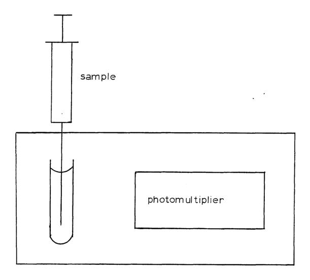
Figure 1-2. Simple system for measurement of CL. Photomultiplier and cuvette containing reagents are mounted in a light-tight housing. The needle of the sample syringe is inserted through a septum.
