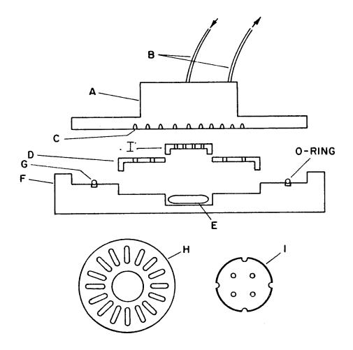
Figure 3-3. Two phase flow cell. A: aluminum spiral channel piece;
