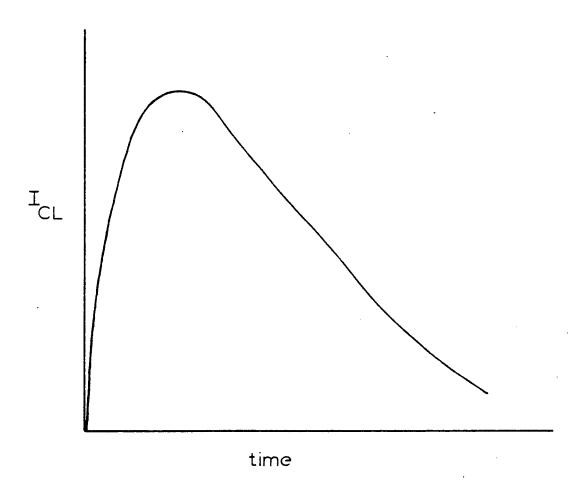
Figure 1-1. Generalized intensity-time curve for a CL reaction.
