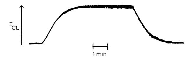
Figure 3-17. Steady state response of bacterial BL in two phase flow system. Sample was  $10^{-5}$   $\underline{\text{M}}$  NADH. Flow rate = 1 mL/min.
