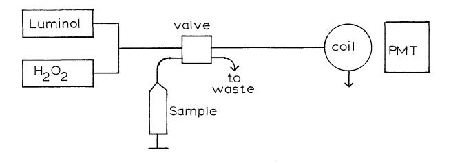
Figure 2-5. FIA system for Cr(III) determination. A two-channel peristaltic pump drove the luminol and  $\rm H_2O_2$  syringes. A separate, single-channel pump drove the sample syringe. The coil of Teflon tubing was mounted flat against the face of the photomultiplier.
