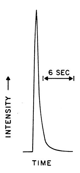
Figure 3-4. Intensity-time response for injection of  $\rm H_2O_2$  into the photometer, with fast kinetics luminol-peroxidase system.
