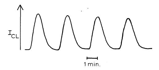
Figure 3-15. Replicate injections of 10<sup>-6</sup> M ATP into two phase flow system operated in flow injection mode. Reagent contained 10 mg/ml apyrase. Sample size was 1.0 mL. Flow rate = 1 mL/min.
