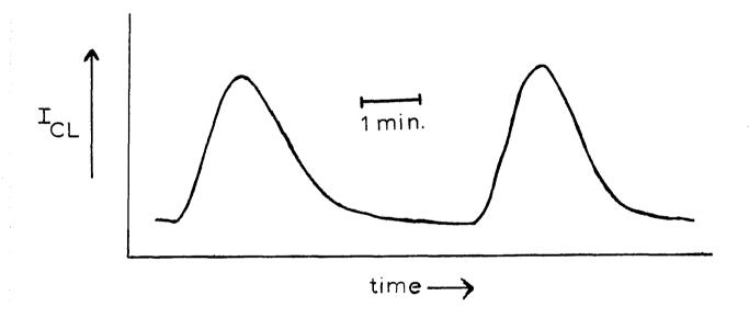
Figure 3-14. Replicate injections of  $10^{-6}$  M ATP into two phase flow system operated in a flow injection mode. Reagent contained 1 mg/mL apyrase. Sample slug size was 1.0 mL. Flow rate = 1 mL/min.
