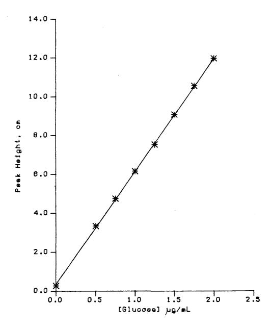
Figure 2-14. Standard curve for glucose in CL-FIA system.
