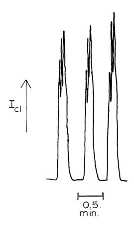
Figure 2-6. Signals for replicate injections of  $10^{-6}$  M Cr<sup>3+</sup> in 0.4 M  $_{12}^{0}$  M  $_{2}^{0}$ , untitrated.
