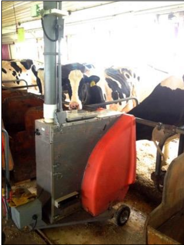
Figure 1. The Greenfeed system mounted on a cart inside the tie stall barn (a) and the use of a heart-rate sensor in cows to determine O 2 pulse (b).
