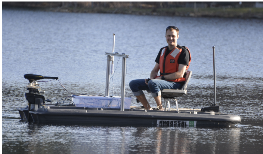
Figure 1.7: Undergraduate ASV3, underway for sonar data collection with the author aboard.
