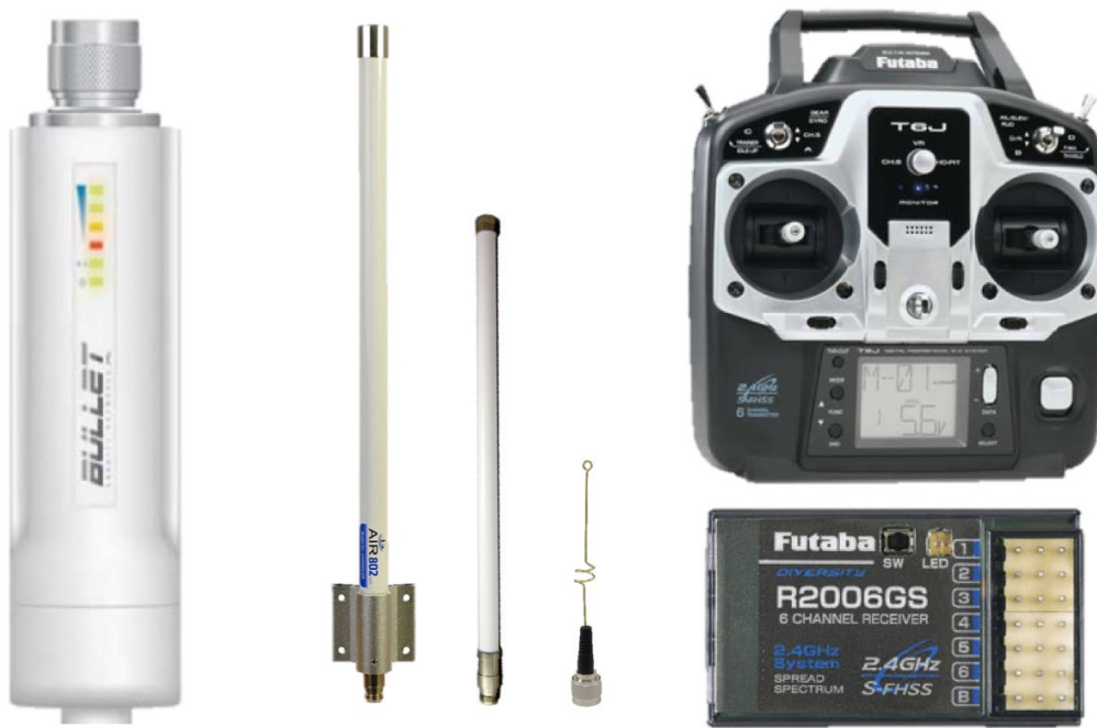
(a) Ubiquiti Bullet BM5HP and 12 dBi, 10 dBi, and 5 dBi antennas. Bullet not to scale with antennas. (b) Futaba 6J and R2006GS
