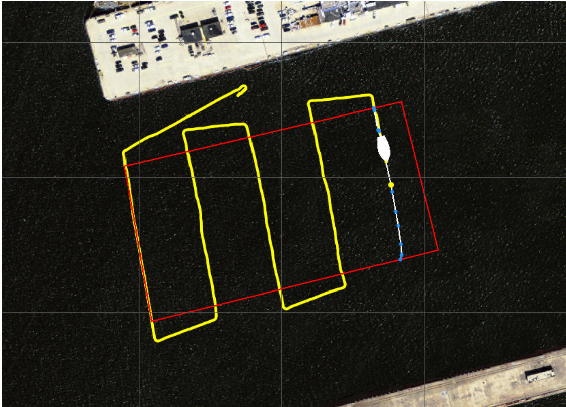
Figure 3.18: MOOS-IvP pMarineViewer monitoring view of automated survey in progress. Operation region shown in red, current survey line in white and vessel track in yellow.
