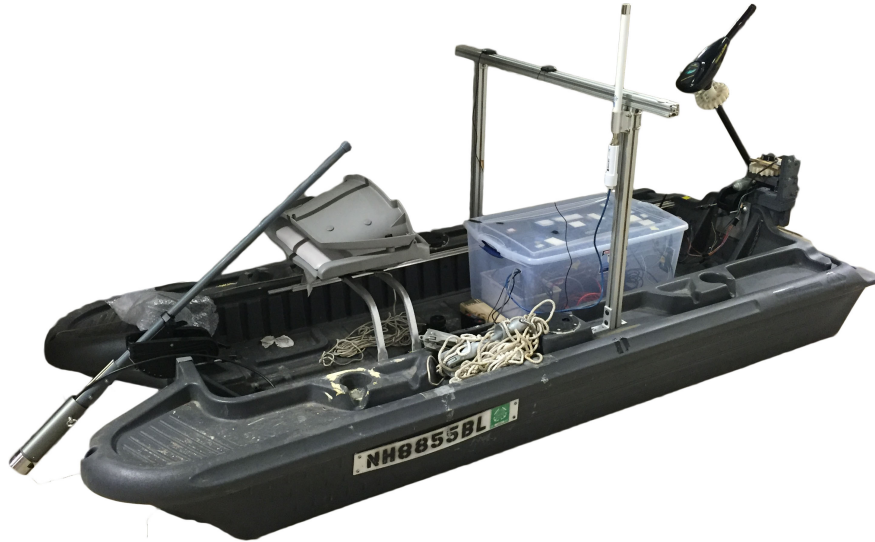
Figure 1.6: Undergraduate ASV3, in storage configuration with propulsion and sonar systems retracted.
