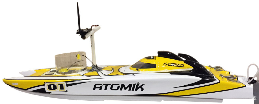
Figure 1.5: Undergraduate ASV2, including mast for antennas.
