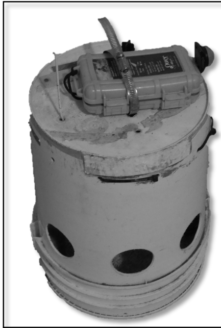
Figure 2.1 A Paul drifter. The GPS unit is placed into the otter box on the top part of the drifter unit, and remains above the water for transmission purposes. The inside of the bucket contains both weights and floatation devices, so that it floats with about \frac{1}{4} of the drifter above water.
