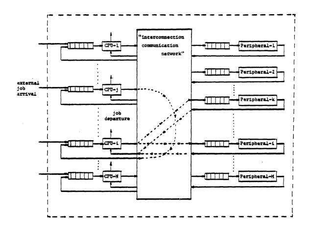
Figure 3-1. Decentralized Control Model for Distributed Systems
