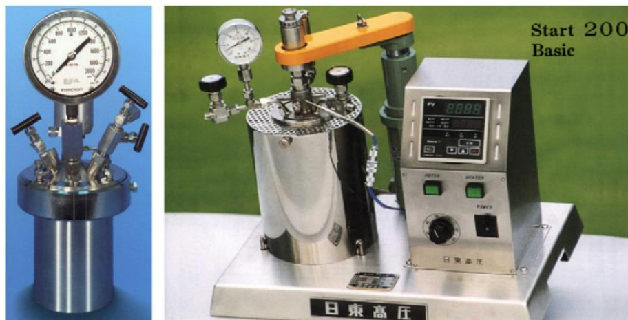
Figure 1.11: Commercially available magnetically stirred steel pressure vessel configured with pressure control and an external pump to control the gas flow [35].
