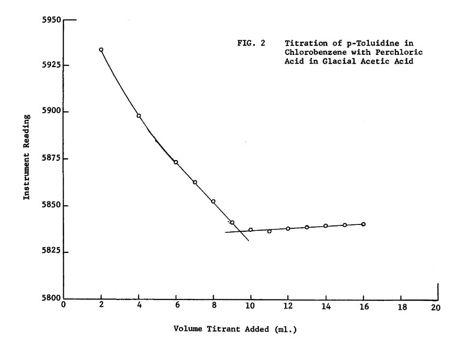
point volume is 9.40 ml. and the shape of the titration curve obtained is " \_\_\_\_ "; i.e., a deformed "V". Looking at the instrument response curve, this would be expected, for the equivalence point volume (9.40 ml.) falls on the fairly "flat" region of the response curve.
