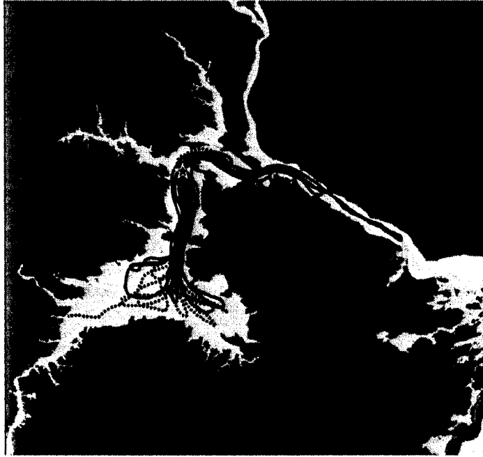
Fig. 7. Spaghetti plots for two ‘Paul’ drifters released in Little Bay (GBE) in July, 2011. Both drifters were at-large over 10 days and were exposed to ~ 20 tidal cycles. This pattern was common in the other drifters we deployed regardless of the time we released them.
