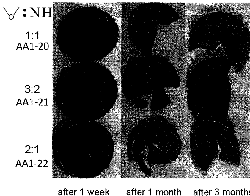
Figure 23. Color change of clear model epoxy matrix with different rigidity mixed with 0.06 wt% of Alizarin Yellow R.
