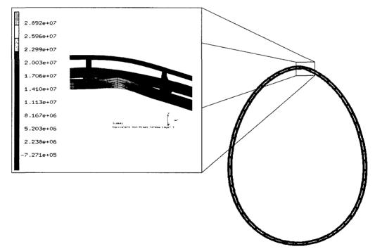
Figure 5.26: The von mises stress distribution on the net pen rim when 53 kN is applied as a distributed
