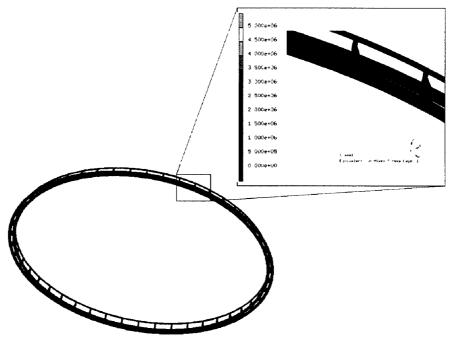
Figure 5.23: Von Mises Stresses in the net pen structure using environmental loading data of 16-may 2004 at 2200 with the 1st load case boundary conditions. The maximum stress occurred on the inside rim in the middle of the distributed loads as seen in Figure 5.18.
