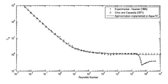
Figure 2.17: Normal drag coefficients for a cylinder. The experimental values are compared to the Choo and Casarella approximation and equation (2.29).
