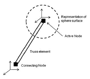
Figure 2.5: The spherical element consists of two nodes: the active node where the mass and characteristics are applied, and the connecting node.
