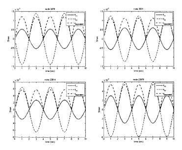
Figure 6.8: The output strain results from the structural analysis of the thin wall pipe under forcing described by equation 6.2.
