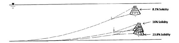
Figure 4.8: Submerged configurations of the OCAT system at 1.5 m/s currents.
