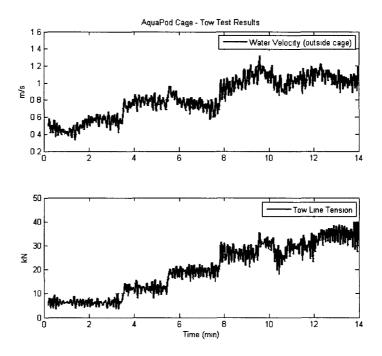
Figure 3.8: Water velocity and load cell readings during the experiment.
