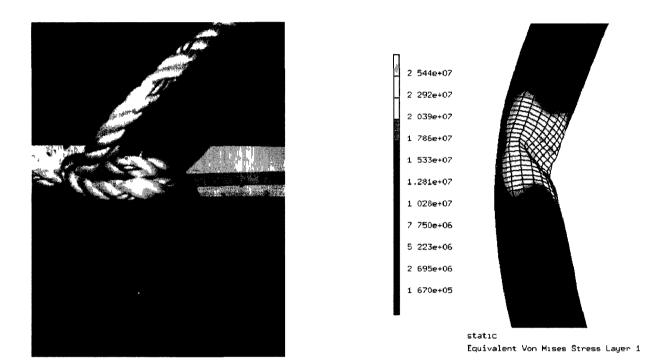
Figure 5.14: A visual comparison between the kinking and localized failure of the circular ring. Note that the yield stress of HDPE is  $2.417 \times 10^7$  Pa.
