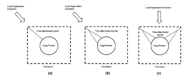
Figure 5.25: The attachment configurations were modeled where the net pen was secured with one (a), two (b) and four (c) point locations.
