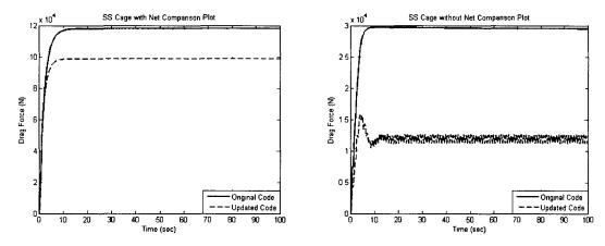
Figure 2.24: The fish cage drag force results under the 2 m/s water velocity. The cage with a net chamber (on left) and without (on right) was analyzed with the original and updated Aqua-FE software.
