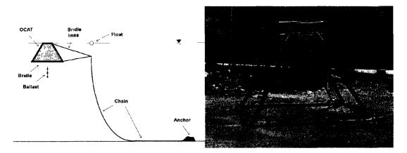
Figure 1.2: A single point moored Ocean Cage Aquaculture Technology (OCAT) fish cage is shown on left. On right: The OCAT is presented without the net chamber for clarity.
