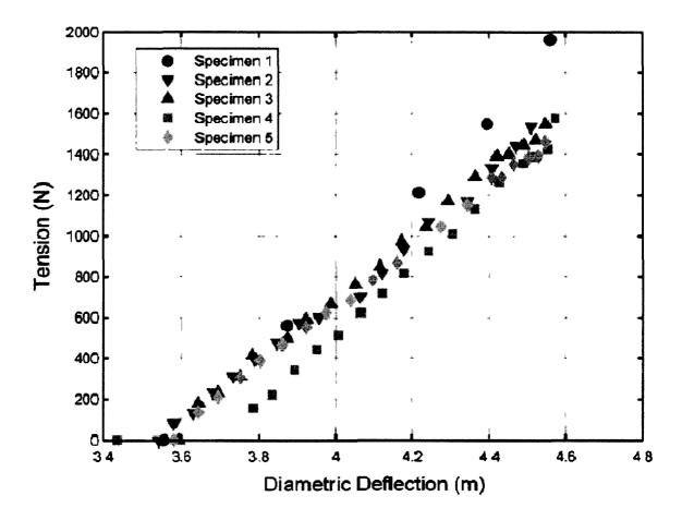
Figure 5.12: The results of the circular ring experiment. The force and associated circular ring diameter are shown. The diametric deflection was measured with a tape measure between the load application point and midpoint between the supporting bridles.
