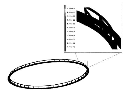
Figure 5.24: Von Mises Stresses in the net pen structure using environmental loading data of 16-may 2004 at 2200 with the 2nd load case boundary conditions. The maximum stress occurred at the SE y-line load application point (maximum y-line tension).
