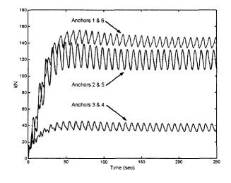
Figure 7.5: Selected mooring line load results using one of the UNH design conditions. Anchors are
