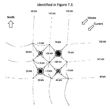
Figure 7.6: The maximum load distribution in the mooring using one of the UNH design conditions. The current and waves are applied from the northeast direction.
