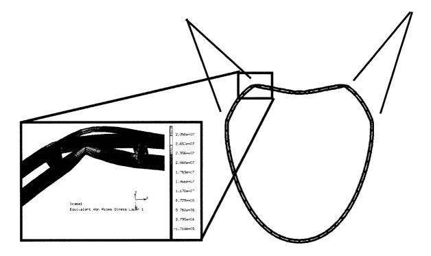
Figure 5.29: The stress distribution on the cage frame when y-lines are moved such they are not longer equally spaced around the cage circumference.
