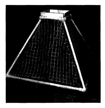
Figure 4.2: 1:10 Froude scale model of the OCAT cage
