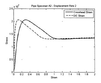
Figure 6.18: The stress-strain curves for a specimen obtained from pipe sample 2 under displacement rate 2. The curves were obtained using the calculated crosshead and DIC measured strains.
