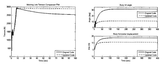
Figure 2.23: The site marker mooring tension and buoy tilt angle under the 2 m/s water velocity. The system was analyzed with the original and updated software.
