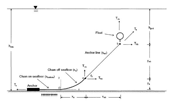
Figure 7.4: Anchor leg definition schematic. Note that the float assembly consists of the float, a length of chain and the rope ring corner connections (not shown).
