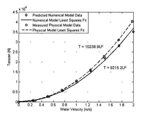
Figure 4 6. Comparison between full scale numerical and (recalculated to full scale) physical model predictions of the drag on the OCAT cage system.
