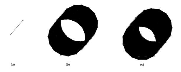
Figure 5.2: Three element types representing the same length of pipe. (a) 2 node line element, (b) 2D shell elements, and (c) 3D brick elements.
