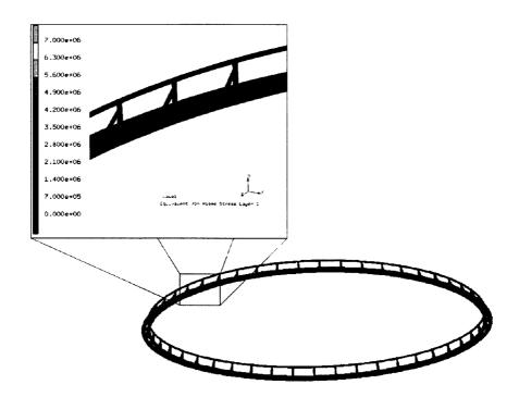
Figure 5.22: Von Mises Stresses in the net pen structure using environmental loading data of 5-may 2004 at 1200 with the 2nd load case boundary conditions. The maximum stress occurred at the SW y-line load application point (maximum y-line tension).
