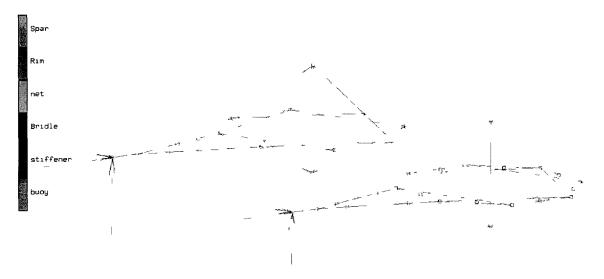
Figure 2.20: FEA models of two SeaStation<sup>™</sup> fish cages were constructed in Aqua-FE. One had a net chamber (lower right), where the second one only had the rims and tensioned stays (upper left).
