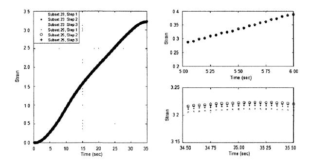
Figure 6.16: Sensitivity test results comparing the strain in a sample from the unused pipe at displacement rate 1, 9.525 x 10<sup>-1</sup> mms<sup>-1</sup> for the 6 load cases. Left: The total specimen strain. Top Right: The strain in the linear elastic region of the specimen. Bottom Right: The strain at the yield stress.
