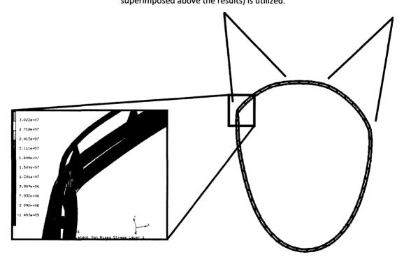
Figure 5.28: The von mises stress distribution on the net pen rim when two, symmetrical y-lines (shown superimposed above the results) are utilized.
