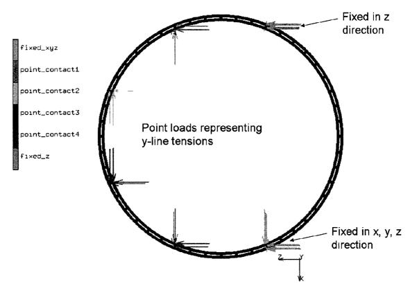
Figure 5.18: The tensions in the mooring line are represented by point loads applied to ½ the pipe circumference and evenly distributed on the inner and outer rims. The two additional bridle line supports (would be present in the "minor arc" of the cage frame), were not taken into consideration for this analysis.
