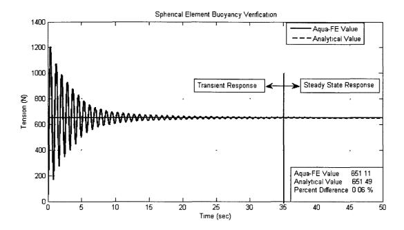
Figure 2.9: The output line tension results. The transient and steady state tension regions are also shown.
