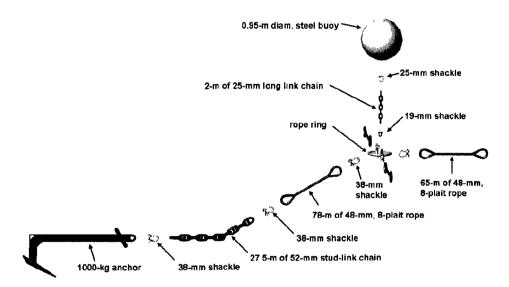
Figure 7.7: Component details of the side grid mooring assembly. Some items are not to drawn to scale.
