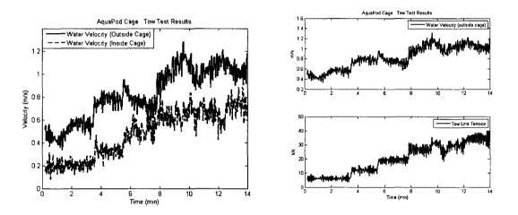
Figure 3.11: The measured water velocity reduction and tow line tension.
