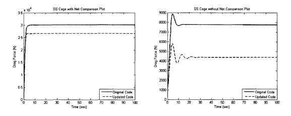
Figure 2.22: The fish cage drag force results under the 1 m/s water velocity. The cage with a net chamber (on left) and without (on right) was analyzed with the original and updated Aqua-FE software.
