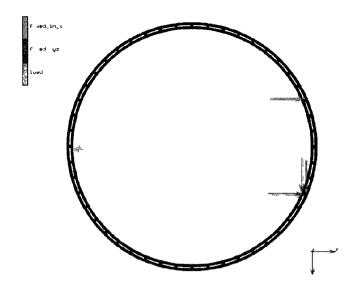
Figure 6.6: The boundary conditions applied to the FEM.
