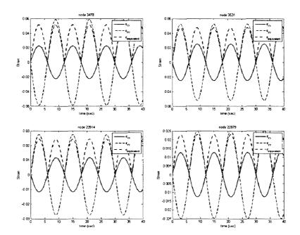
Figure 6.9: The output strain results from the structural analysis of the thin wall pipe under forcing described by equation 6.3.
