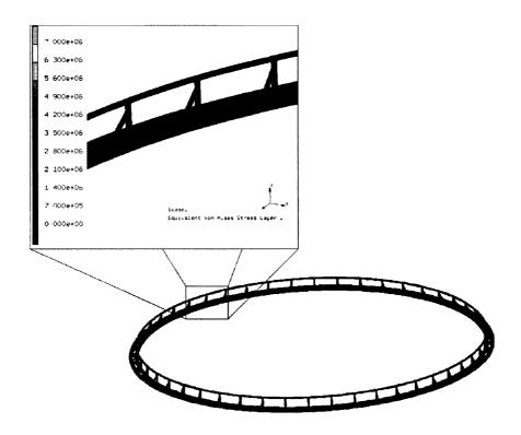
Figure 5.21: Von Mises Stresses in the net pen structure using environmental loading data of 5-may 2004 at 1200 with the 1st load case boundary conditions. The maximum stress occurred on the inside rim in the middle of the distributed loads as seen in Figure 5.18.
