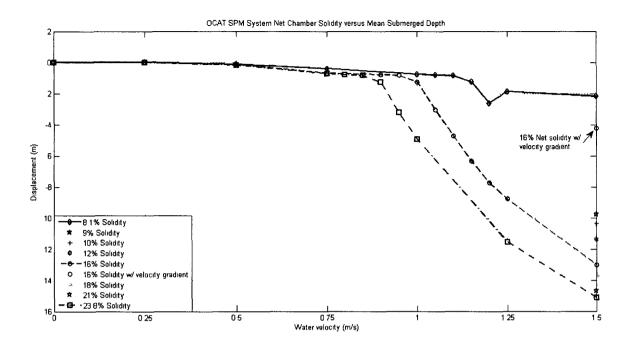
Figure 4.7: Submergence depth of the OCAT system for various netting solidities and water velocities. Note that the 9%, 10%, 12%, 16% with velocity gradient, 18% and 21% solidities were only examined at 1.5 m/s.
