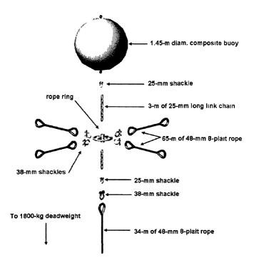
Figure 7.9: Component details of the center grid mooring assembly. Some items are not to drawn to scale. The center node is held down by a 1800 kg steel deadweight.
