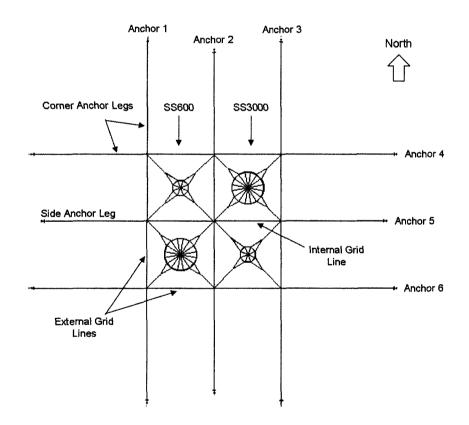
Figure 7.3: A top view of the submerged grid mooring system. It consisted of 8 corner anchor legs, 4 side anchor legs, 1 center anchor line, 12 grid lines, and 16 bridle lines. The anchors on the north and east sides are numbered for load identification.
