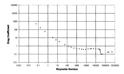
Figure 2.2: Dependence of drag coefficient of a sphere on Reynolds Number. Obtained from Donley, 1991.
