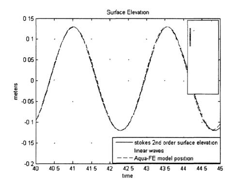
Figure 2.15: The surface wave elevation and Aqua-Fe model position.
