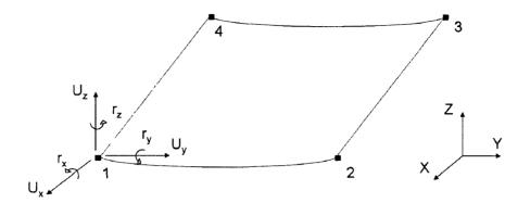
Figure 5.8: The four-node shell element with 6 degrees of freedom per node.
