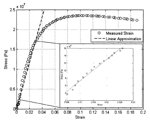
Figure 6.19: The stress-strain curve obtained from tensile testing of HDPE specimen 1 of Pipe A1.
