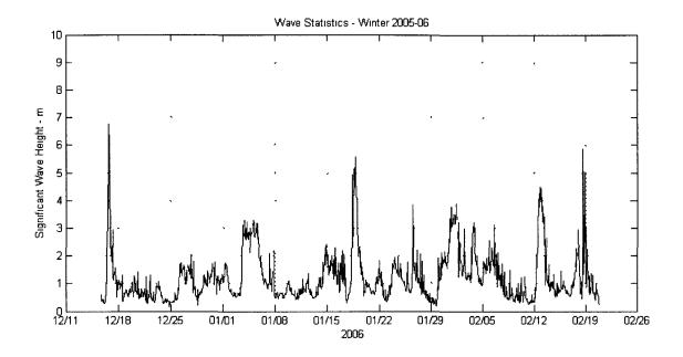
Figure 7.19: Typical winter storm waves in 2005-2006 with significant wave heights of 4 to 6 m.
