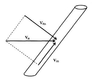
Figure 2.1: Relative fluid velocity components acting on a cylindrical element. The n and t subscripts represent the normal and tangential directions, respectively.
