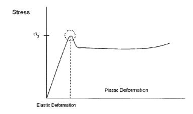
$\label{eq:Strain} Figure 6.14: The tensile strength at yielding, \sigma_y, was obtained for each specimen.$
