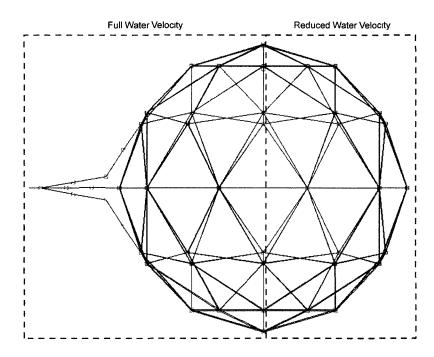
Figure 3.13: The full ambient water velocity was applied to the front half of the cage system. The water velocities measured inside the cage were applied to the aft portions of the model.
