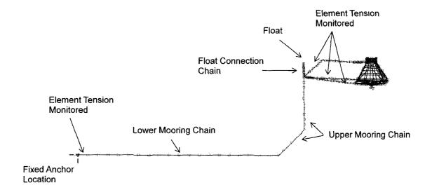
Figure 4.5: Finite element model of the full OCAT cage and single point mooring system. The cage and bridle line components are similar to those shown in Figure 6. The tensions within four elements were recorded to provide mooring component tension.
