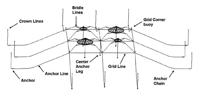
Figure 7.2: An isometric view of the submerged 4-cage grid system.
