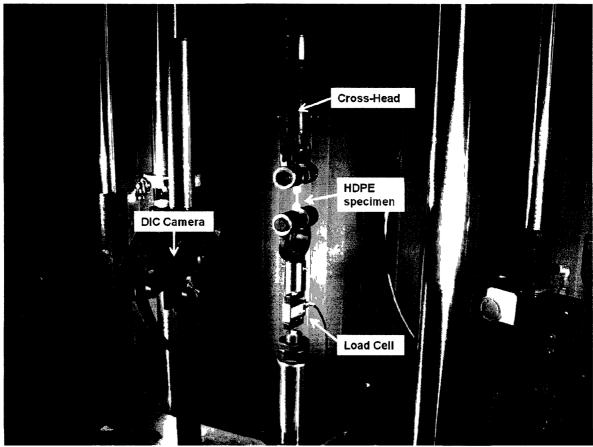
Figure 6.11: The test set-up of the experiments performed on the Instron tensile testing machine. The force straining the HDPE specimen was recorded from the load cell. The specimens strain was calculated from the Instron cross head movement and DIC measurements
