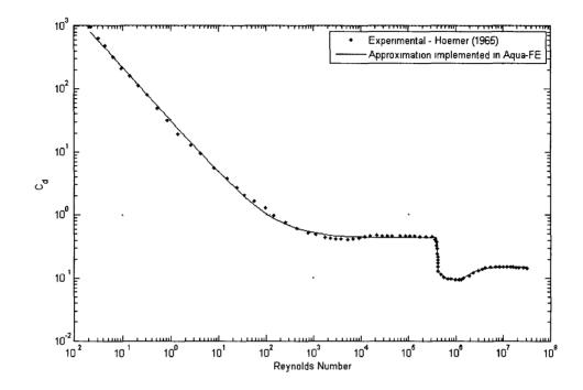
Figure 2.4: Drag coefficients for a sphere. The experimental values are compared to equation (2.10). Experimental values were obtained from Hoerner (1965) and numerical approximation by DeCew et al., 2010.
