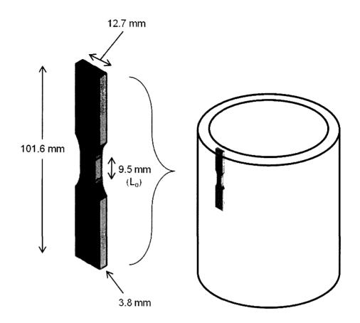
Figure 6.10: Twenty specimens were fabricated from each pipe segment. The samples were 101.6 mm long, 12.7 mm wide and 3.8 mm thick. The testing gage length, L<sub>o</sub>, was 9.5 mm.
