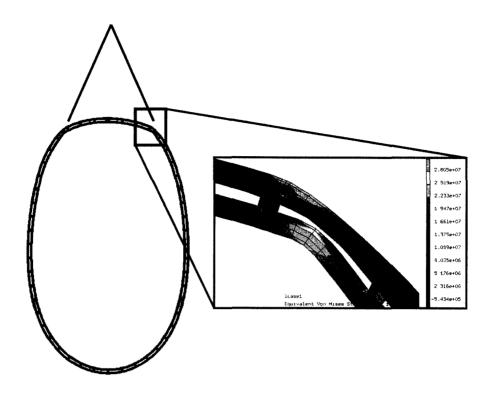
Figure 5.27: The von mises stress distribution on the net pen rim when one full y-line (shown superimposed above the results) is utilized.
