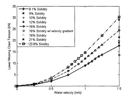
Figure 4.9: Variation of the mooring chain tension with water velocity for different net solidities.
