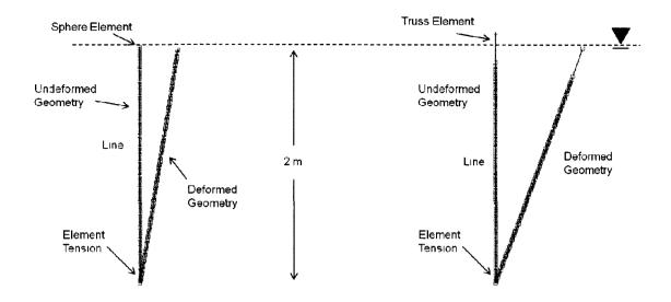
Figure 2.10: The truss and spherical floats were modeled using similar mooring lines in Aqua-FE. The deformed geometry is shown for the 1 m/s water velocity as an example.
