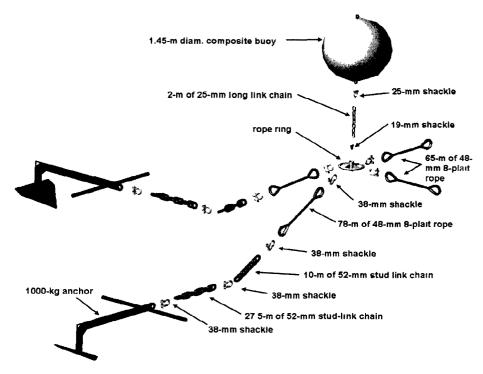
Figure 7.8: Component details of the corner grid mooring assembly. Some items are not to drawn to scale.
