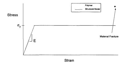
Figure 5.9: Approximation of polymer material behavior by linearly elastic – perfectly plastic curve.
