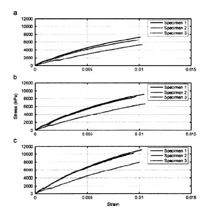
Figure 5.7: Stress strain data results when loaded at 0.0127mm/s, 0.127 mm/s and 1.27 mm/s.
