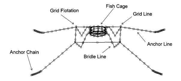
Figure 6.2: The Aqua-FE cage-grid mooring system model. A gravity fish cage was placed in a submerged grid, 18 meters below the surface in 45 meters of water. The lower ends of the anchor chain were fixed points.
