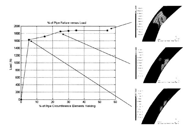
Figure 5.15: The load versus percentage of pipe circumference element failure. The progression of stress contours using the localized failure technique is also shown.
