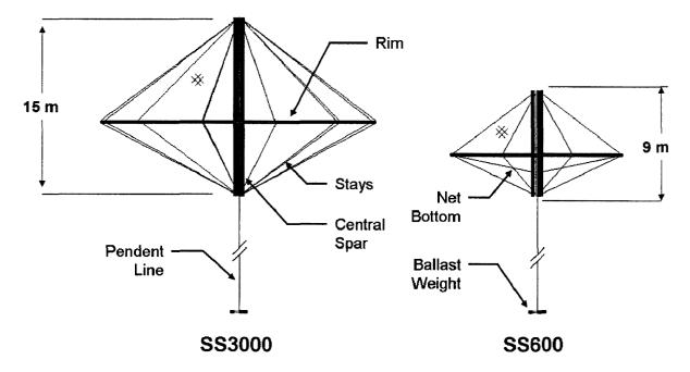
Figure 7.1: The SS600 and SS3000 cages each consist of a central spar and rim held together with tensioned stays. The spar on the SS600 has a length of 9 meters, while the spar on the SS3000 is about 15 meters. The nominal rim diameter of the SS600 is 15 meters, while on the SS3000 it is 25 meters. Each cage incorporates a ballast weight suspended with a pendent line from the spar weighing 19 and 53 kN (dry) for the SS600 and the SS3000 cages, respectively.
