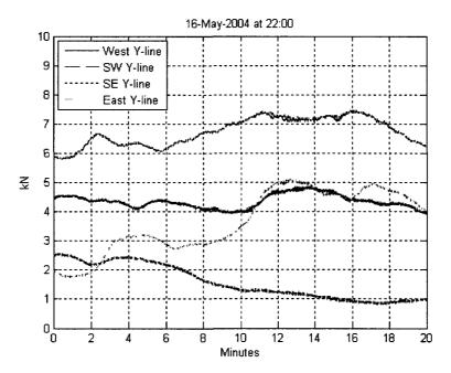
Figure 5.20: The tensions in the y-lines measured on 16-may-2004 at 2200 UTC.
