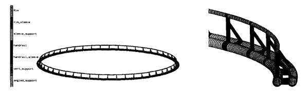
Figure 6.5: The FEM constructed in MSC.MARC/Mentat. The full rim is shown on left, a portion of the mesh on right.
