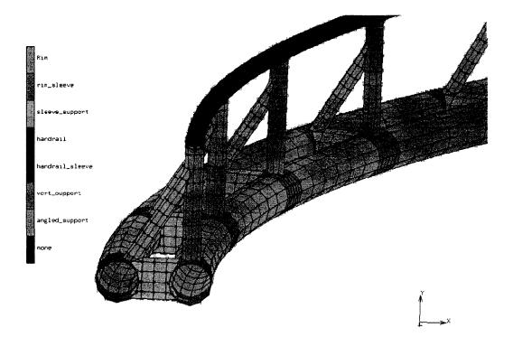
Figure 5.16: An FEM model of a portion of the surface rings used in a net pen.
