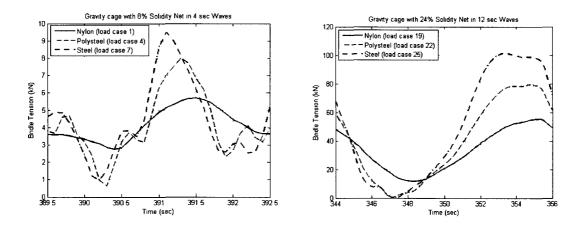
Figure 6.4: The output bridle line tension results with 2 net solidities under two regular wave regimes. The 8% solidity net chamber in 4 second, 1.66 meter waves (left) and 24% solidity in 12 second, 13.5 meter waves (right).
