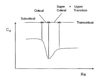
Figure 2 3 · A schematic of the change of the drag force in the critical range of Reynolds numbers. Adopted from "Hydrodynamics around cylinder structures" by M Sumar and J Fredsoe.
