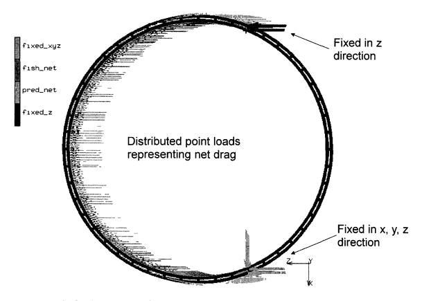
Figure 5.17: The first load case: the drag was assumed to be evenly distributed over "major arc" the inner and outer rims. The two additional bridle line supports (would be present in the "minor arc" of the cage frame), were not taken into consideration for this analysis.
