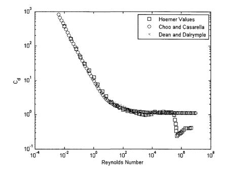
Figure 2.16: Coefficient of Drag versus Reynolds for a smooth circular cylinder. Choo and Casarella approximations work well at Re number below  $3 \times 10^5$ , however neglect the reduction in coefficient of drag in critical flow regions.
