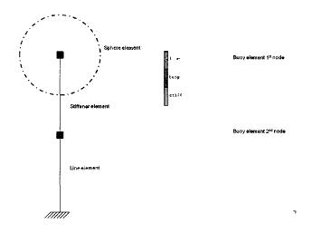
Figure 2.8: A buoyant spherical float placed at the end of a line (left) was modeled in Aqua-FE (right). Note that the buoy and stiffener elements overlay each other in the Aqua-FE model.
