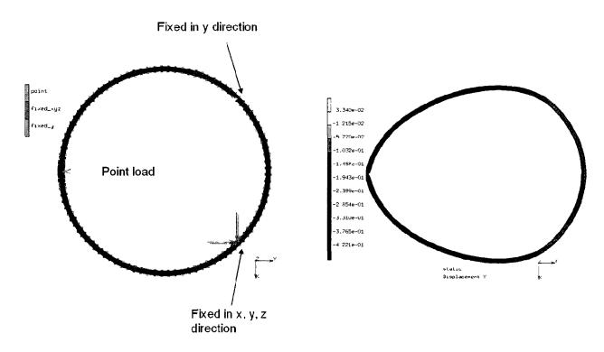
Figure 5.13: Using the values in Table 5.2, FEM calculations were performed to simulate the weathered ring experiments. Note that the ropes pull inward, present in the laboratory experiment, was not replicated in the FEM. The displacement, in meters, in the horizontal position (Y) is shown along the deformed geometry (right).
