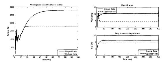
Figure 2.21: The site marker mooring tension and buoy tilt angle under the 1 m/s water velocity. The system was analyzed with the original and updated software.
