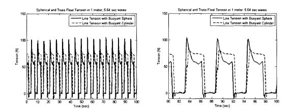
Figure 2.12: Element tension results of the model under 1 meter, 5.64 second waves. The full time series is shown on left, a 20 second section of the data is presented on right.
