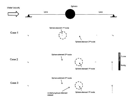
Figure 2.6: A sphere was placed in line of a rope and analyzed under a constant with depth water velocity (top). The cases were investigated where the sphere's active node was moved and the underlying elements connectivity reversed.
