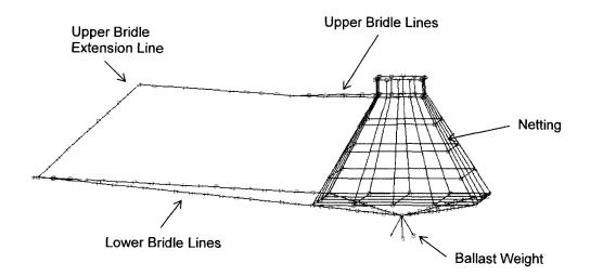
Figure 4.4: Finite element model of the cage and bridle line components.
