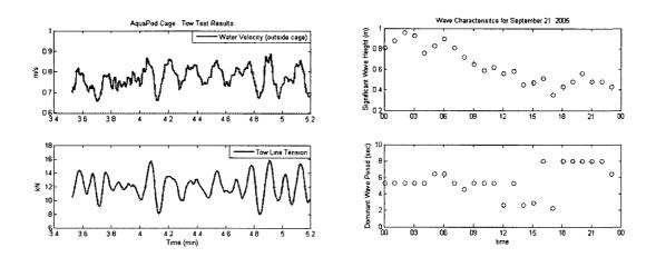
Figure 3.9: A subset of load cell tension measurements and wave characteristics present of the day of the tow. The tow test was initiated at 16:00 EST.
