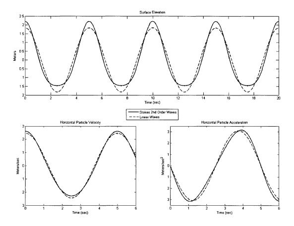
Figure 2.14: The Stokes 2nd order wave surface elevation (top), vertical water particle velocity (bottom left) and acceleration (bottom right) compared Airy waves. The waves had the following properties: T = 5 seconds, H = 3.654 meters, h = 10 meters, L = 36.54 meters, H/L = 1/10.
