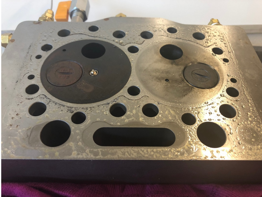
Figure 4.9: Cylinder Head exposed to Combustion Chamber
