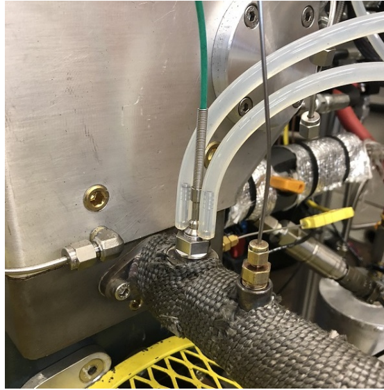
Figure 2.7: Exhaust Pressure Transducer Location
