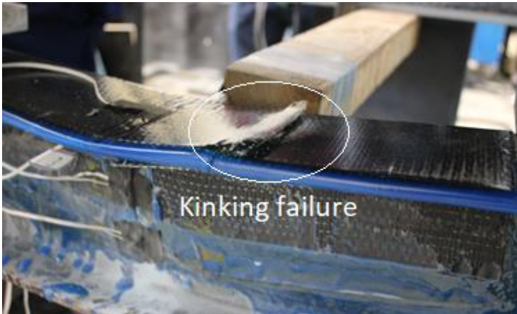
Figure 3.11: Kinking along the stress concentration line
