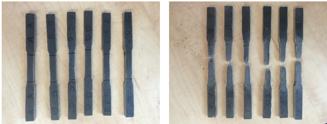
Figure 1.16: Steel specimens before and after testing
