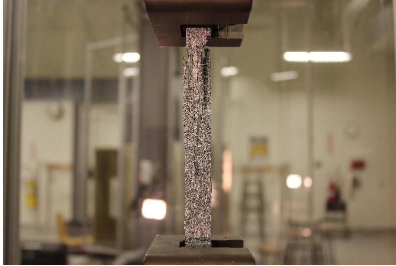
Figure 1.14: Test setup for tension test
