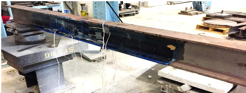
Figure 2.10: Photo of the final rehabilitation scheme with strain gauge
