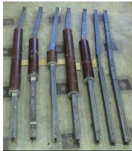
Figure 1.5: Failure type of Specimens (Liu et al)
