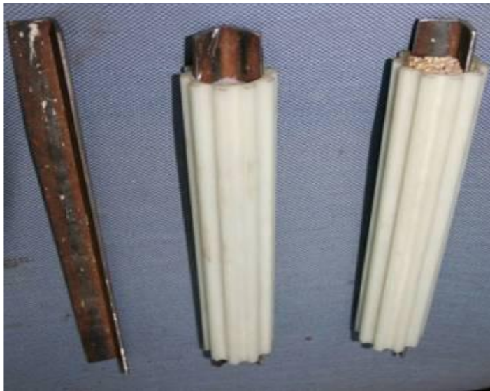
Figure 1.6: Control specimen along with two types of repair (Feng et al.)
