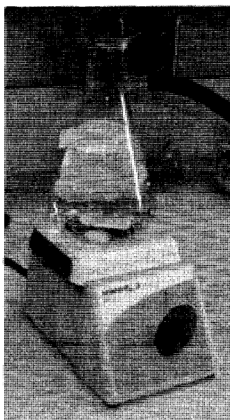
Photo 2.1 Distilled water was agitated under vacuum using a magnetic stirrer to remove CO 2 and O 2 from the solution.
