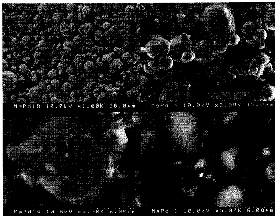
Figure 3.1 Scanning electron micrographs of the Mg/Pd powder (supplied by NASA). Bright spot, as shown by the letter “A”, indicates Pd particles.
