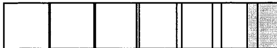
Figure A.1. A GBoundsIterator problem caused by floating point error. The last shaded square should not actually be in the iteration.
