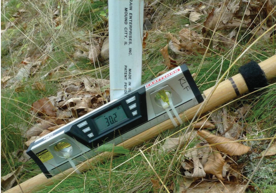
Figure 25. Digital level in use measuring terrain slope.
