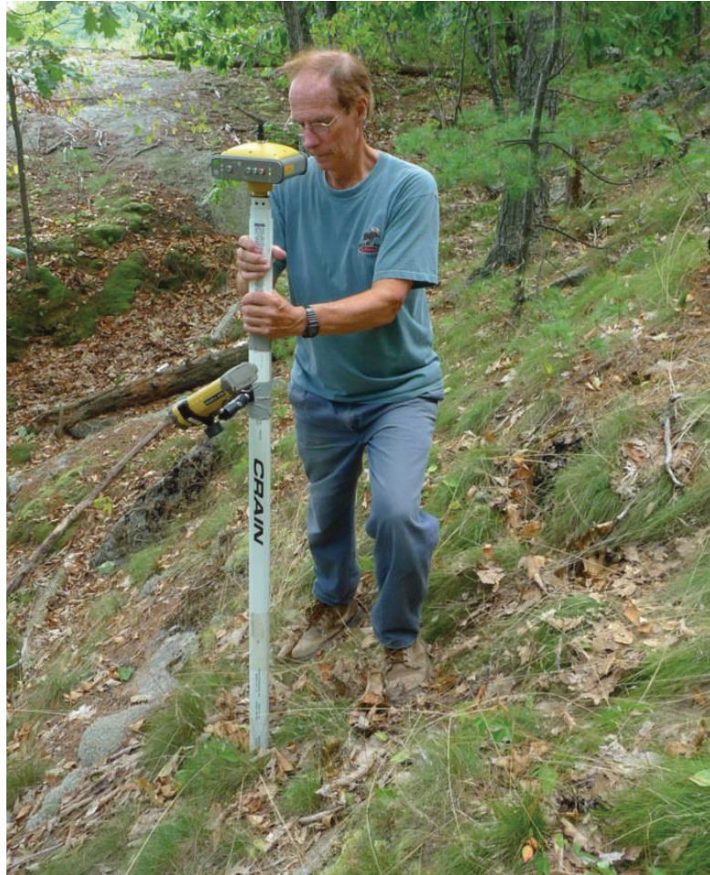
Figure 26. ALTM ground strike location on moderately sloping terrain.
