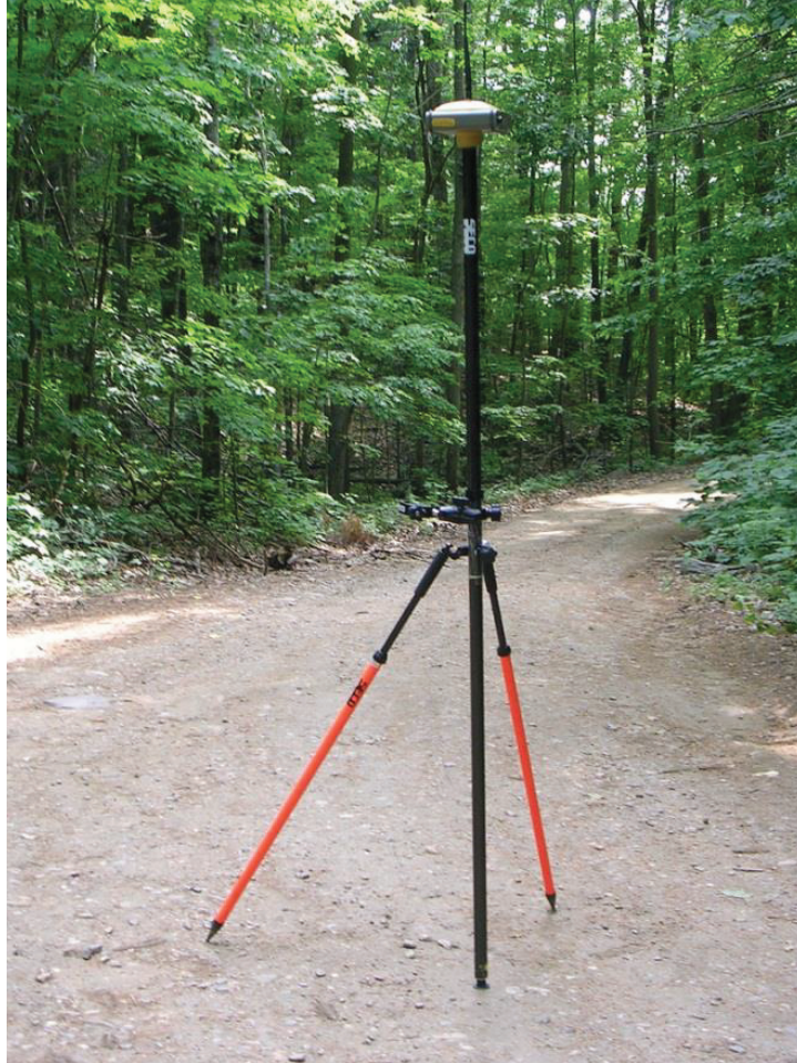
Figure 22. GNSS receiver establishing a horizontal position for orientation of reference points to ALTM ground strikes.
