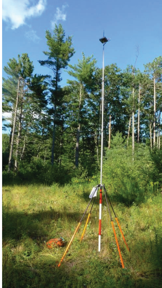
Figure 23. Typical configuration of GNSS base receiver stationed at a control point.
