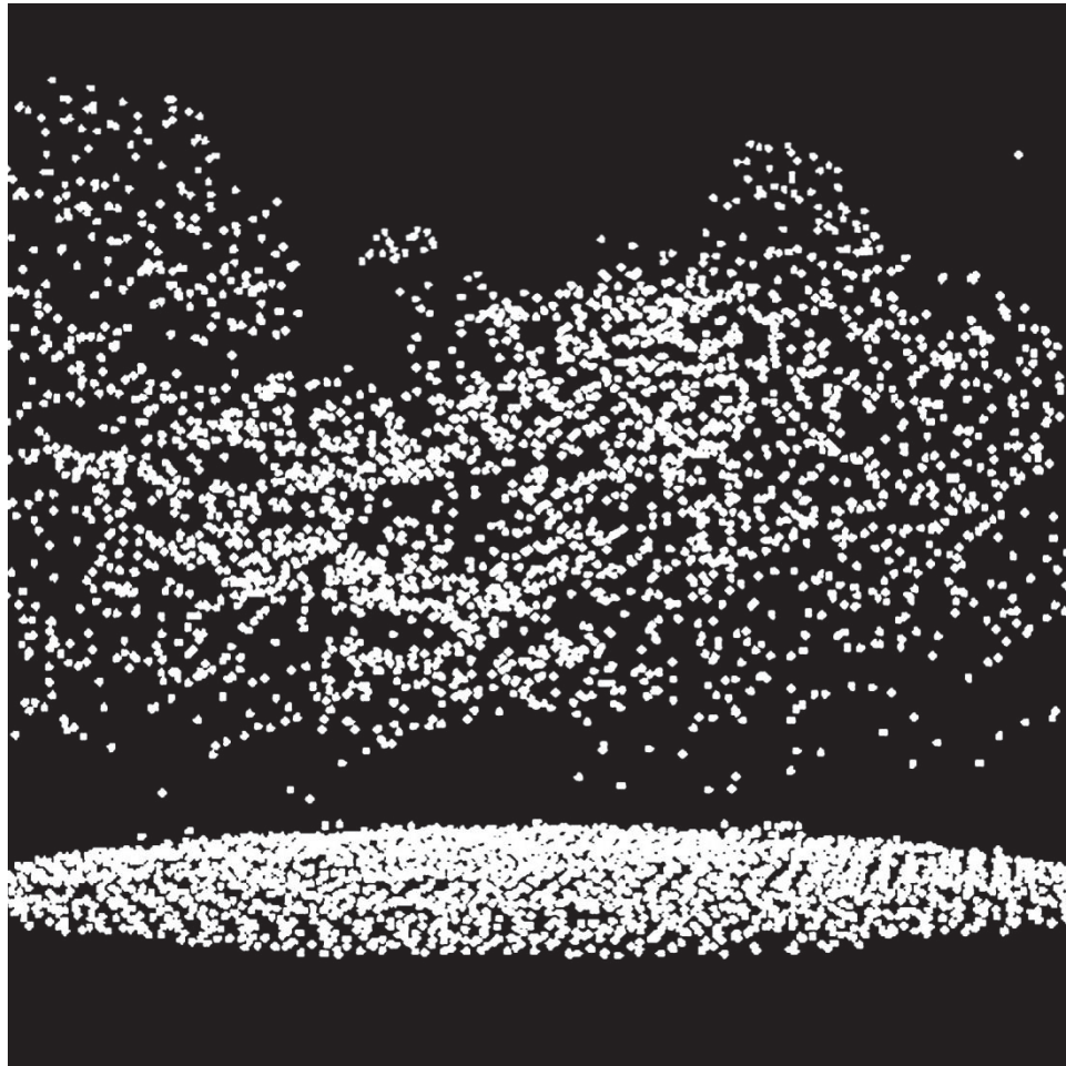
Figure 2. ALTM point cloud created by a discrete pulse system.
