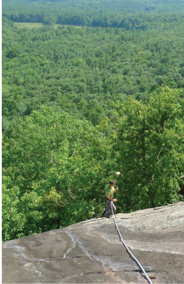
Figure 27. ALTM ground strike location on steeply sloping terrain.
