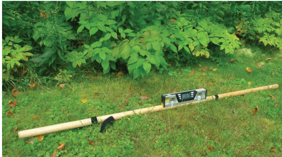
Figure 24. Digital carpenter's level attached to 1.62 m long wooden dowel.
