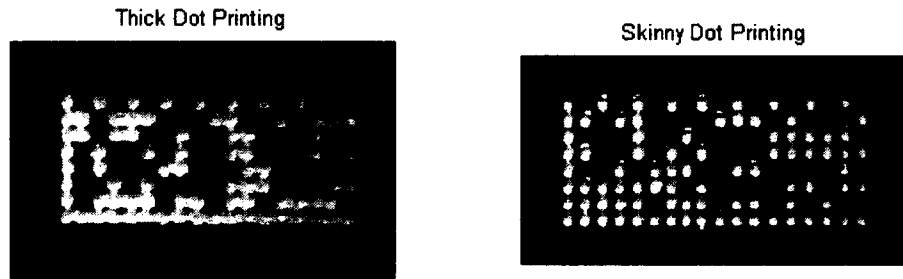
Figure 3.14: Example of Two Data Matrix Printing Types
