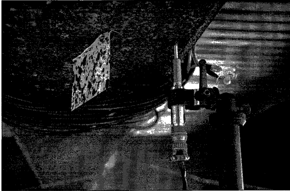
Figure 3 - LVDTs were used during verification testing to ensure the accuracy of DIC measurements.
