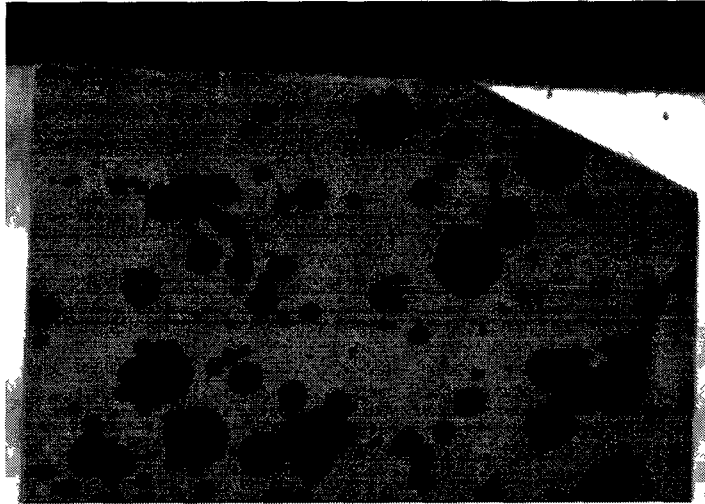
Figure 47 - An ineffective speckle pattern (south span of girder 6).
