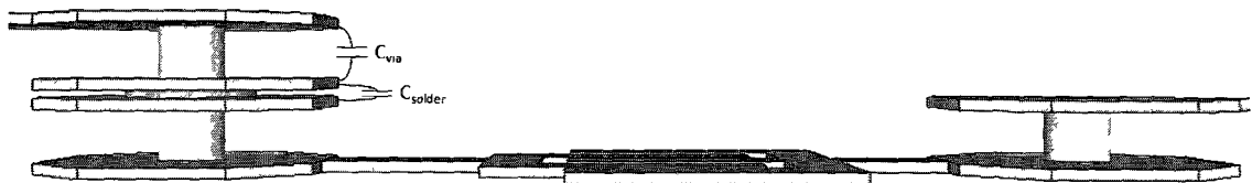
Figure 4.8 - Side View of assembly with associated capacitance
