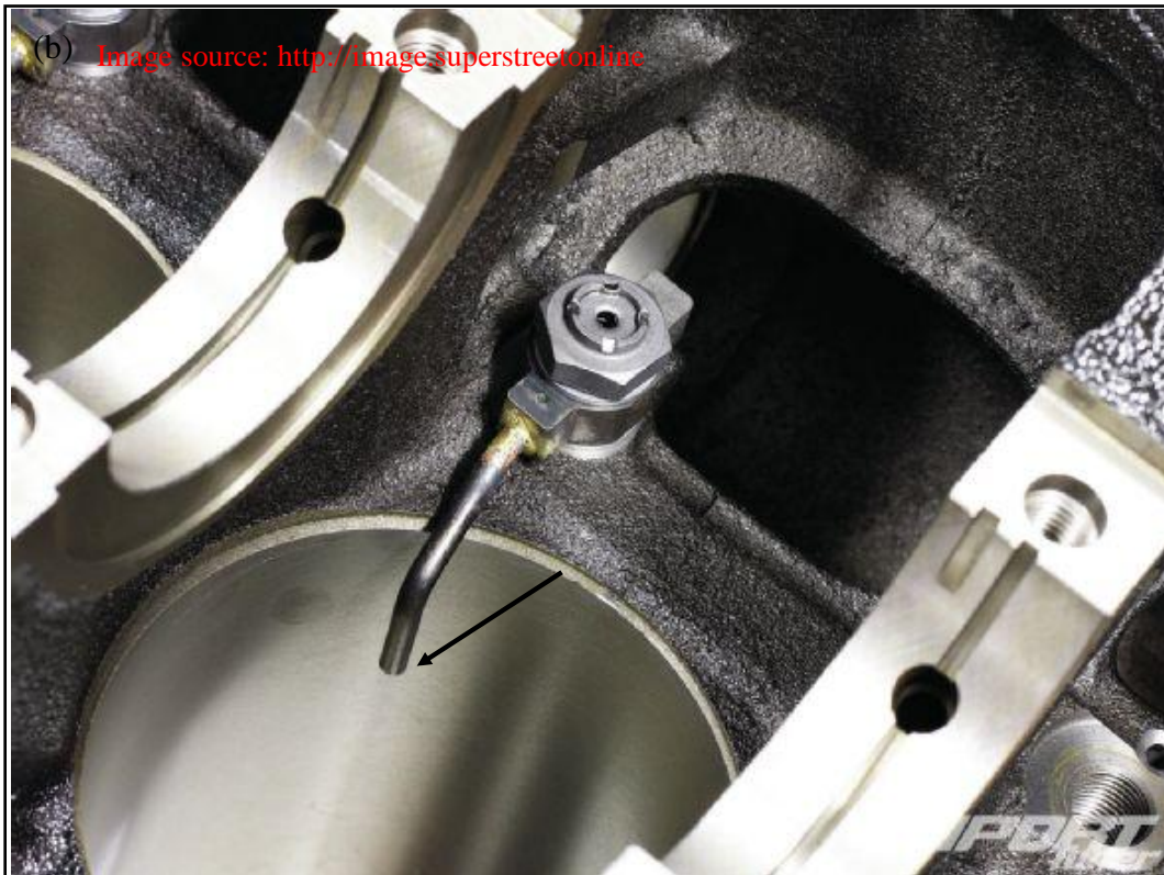
Fig. 1.1 (a) Image of the turbulent jet used as effluents mixing in a river (b) oil squirter assembly for piston cooling
