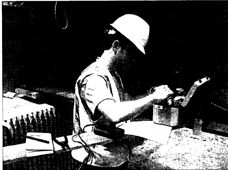
Figure 42. A researcher measures strain using the P3500 for calibration to iSite strain readings
