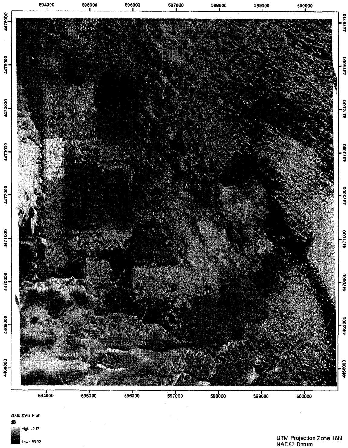
Figure B.3 - 2006 backscatter mosaic assembled with Geocoder with AVG Flat.
