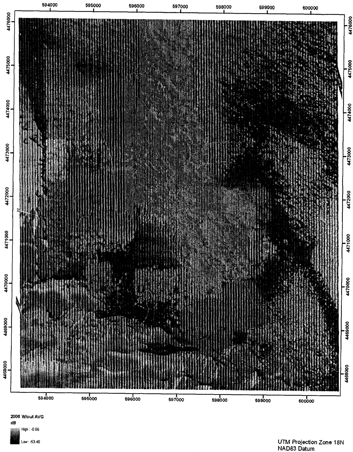
Figure B.1 - 2006 backscatter mosaic assembled with Geocoder without any AVG. The angular response of the sediment makes interpretation of the backscatter mosaic relatively difficult.
